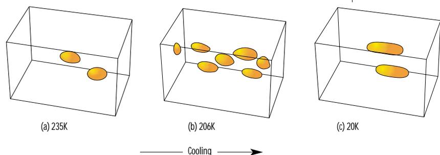
A 3D representation of the neutron scattering peaks as the crystal of the ferromagnetic shape memory alloy is cooled through the martensitic transition
