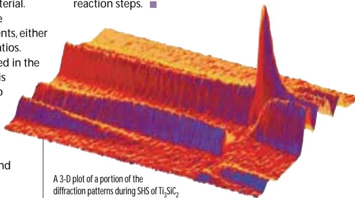
A 3-D plot of a portion of the diffraction patterns during SHS of  $\text{Ti}_3\text{SiC}_2$  as the reaction progresses (left to right)
