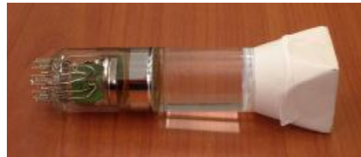
GS10 detector developed by LPC ( ^6\text{Li} doped)
