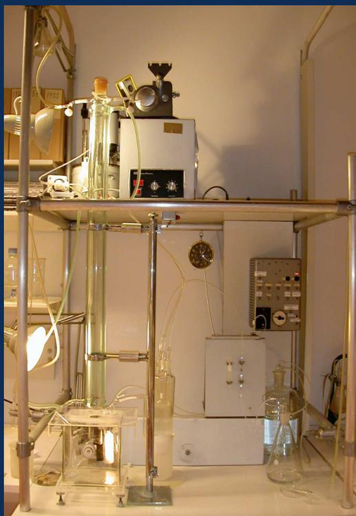
The wet spinning apparatus designed by Allan Rupprecht
