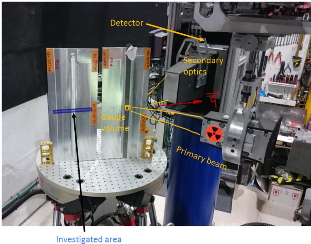
Figure 1 Set-up for measurements in two test welds at the same time. The primary beam is shaped by two radial focussing collimators. A third collimator (secondary optics) in front of the detector defines the third dimension of the gauge volume. The scattering vector  $q$  indicates the investigated strain component. In this specific geometry it is the transversal one. The distance between beam optics and samples is about 400 mm, leaving room for sample movements.
