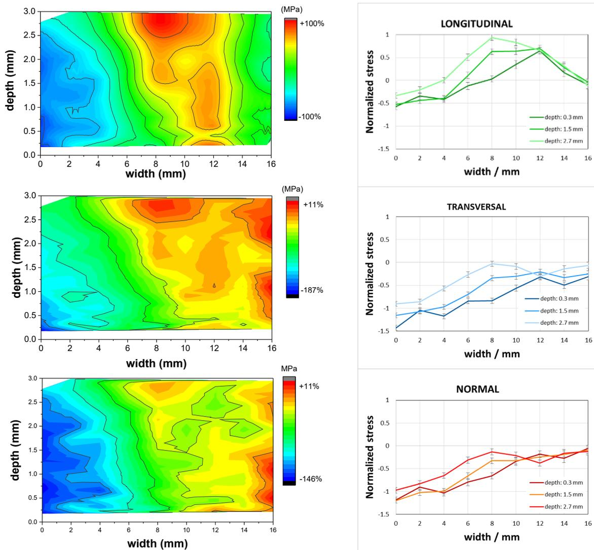
Figure 2 left: Residual stress 2D mapping of longitudinal, transversal and normal components. Right: corresponding profiles at depths of 0.3, 1.5 and 2.7 mm. The weld seam is at 9 mm.
