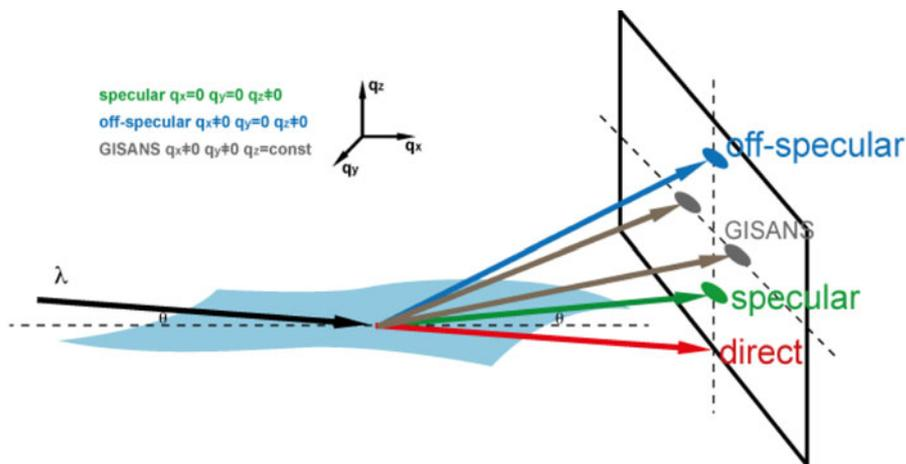
**Fig. 2.** Simple schematic of the geometry of scattering techniques from surfaces.  $\lambda$  is the wavelength of the incoming beam and  $\theta$  the angle.
