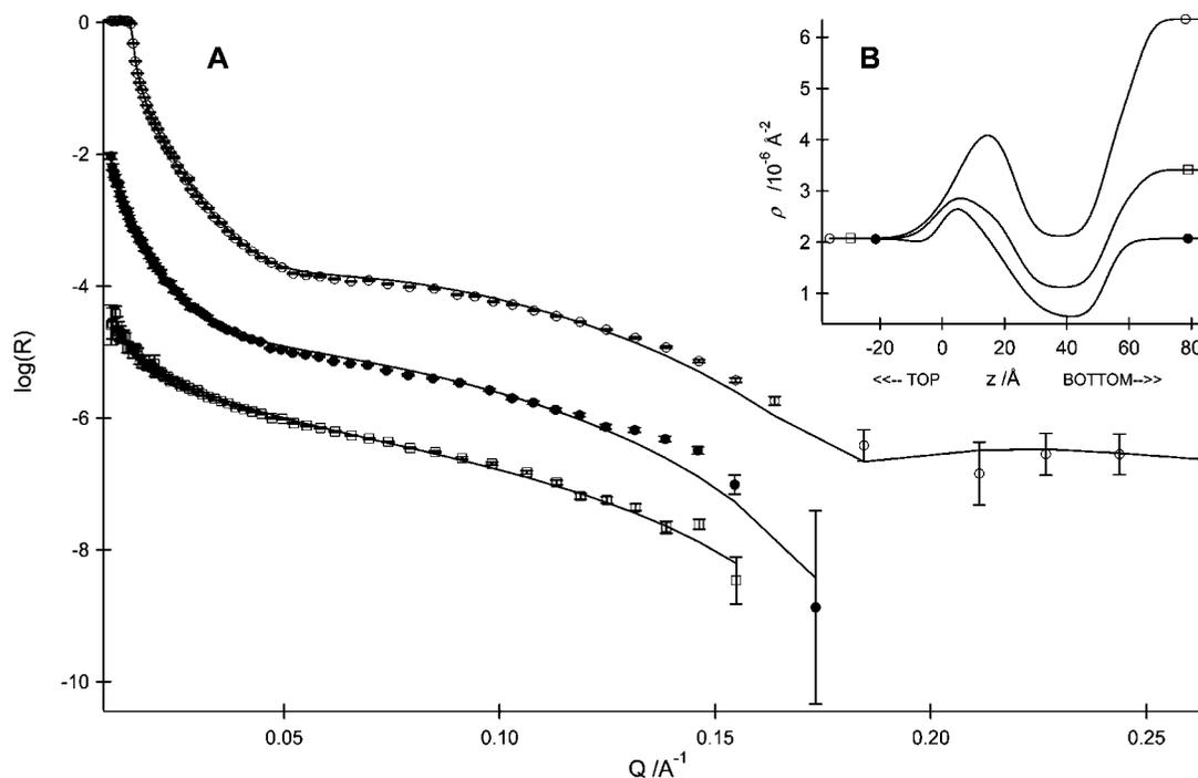
**Figure 2.** DOPC bilayer containing 10% POPS deposited at 20 mN/m. (A) Reflectivity data with D<sub>2</sub>O (○), SiMW (◆), and SiO<sub>2</sub>MW (□) solvents. For clarity, the reflectivity curves are offset by -1 on the y axis.
