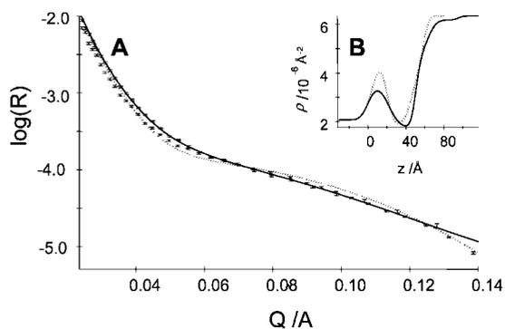
**Figure 5.** DOPC bilayer containing 20% POPS deposited at 20 mN/m. (A) Reflectivity data and (B) SLD profiles for the bilayer before (•••) and after (—) cyt c addition. The solvent used was D<sub>2</sub>O.
