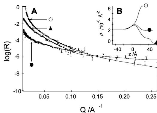
**Figure 6.** Bare silicon substrate. (A) Reflectivity data with D<sub>2</sub>O (○) and SiMW (●) and after cyt *c* addition in H<sub>2</sub>O (▲). (B) Corresponding SLD profiles.
