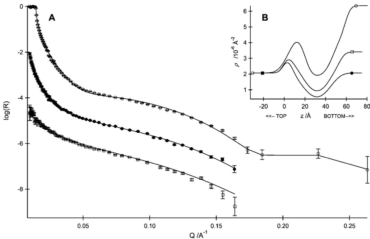
**Figure 3.** DOPC bilayer containing 20% POPS deposited at 20 mN/m. (A) Reflectivity data with D<sub>2</sub>O (○), SiMW (●), and SiO<sub>2</sub>MW (□) solvents. For clarity, the reflectivity curves are offset by -1 on the y axis. (B) SLD profile used to fit the data.
