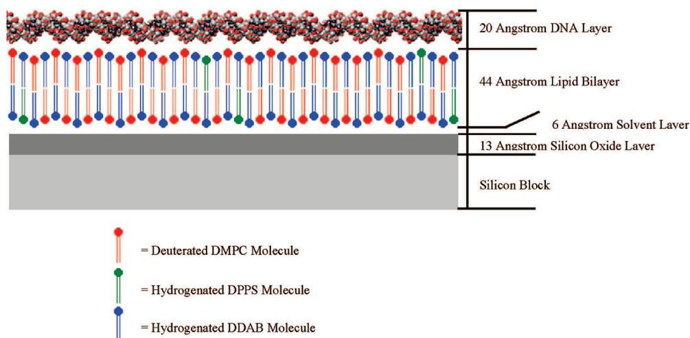
**Figure 5.** Interpretation of the model parameters, described in Table 4, used to fit the neutron reflectivity curves (Figure 4) collected for a model membrane exposed for 5 days to *h*-DDAB/DNA lipoplexes.
