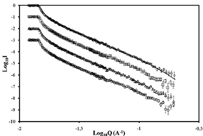
**Figure 1.** Clean silicon surface characterized with D<sub>2</sub>O used as the solvent ( $\diamond$ ) and then exposed to *h*-DDAB/DNA complexes for 2 ( $\square$ ), 4 ( $\Delta$ ), and 6 h ( $\circ$ ). The solid line represents the fit to the surface of the bare silicon block. Data are offset for reasons of clarity.
