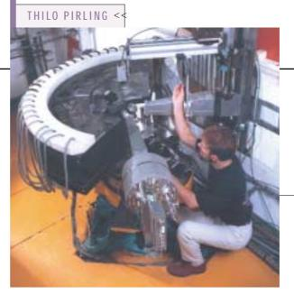
Thilo Pirling aligning the neutron strain imaging instrument with a cog as a sample
