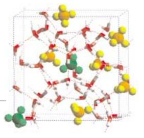
The structure of methane hydrate. Methane molecules occupying small and large cages are shown in green and yellow respectively
