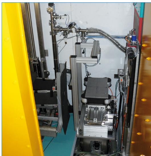
**Figure 2:** Sample area: The goniometer is visible on top of the vertical translation rig. The yellow lead door is closed during measurements.
