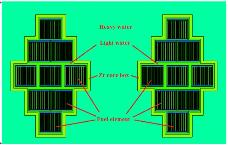
The core consists of total 18 fuel elements which are evenly distributed into two horizontal split regions.
