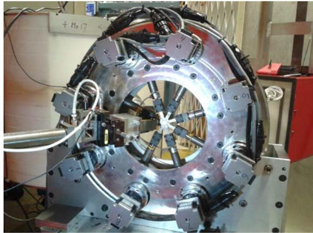
Eight arm multi-directional straining device with 10 kN load capacity.
