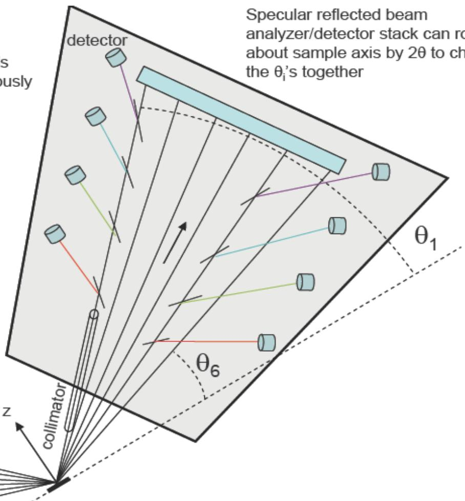
Sample can rotate about its axis (out of the page) by  $\theta$  to change  $\theta_i$ 's together
