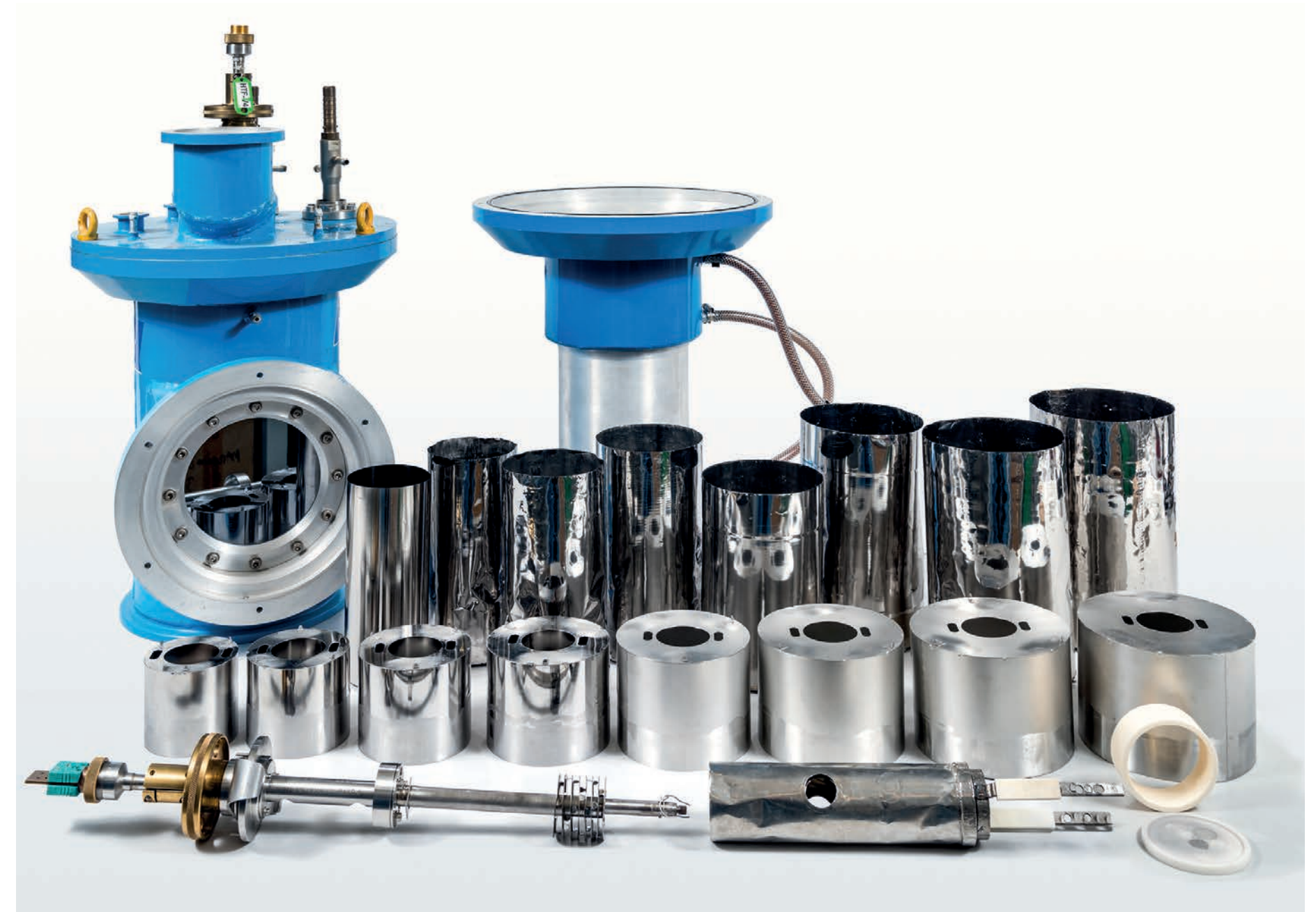
Blue furnace disassembled showing the series of heat shields, the heating elements and a standard sample stick.
