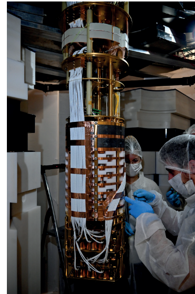
Figure 1: Heart of the cryostat: 18 copper-encased cryogenic calorimeters are installed on the 10 mK stage below the inner shielding of HDPE, copper and lead at the 1 K stage. The inner veto is installed on the 4 K stage. The outer shielding is visible in the background.
