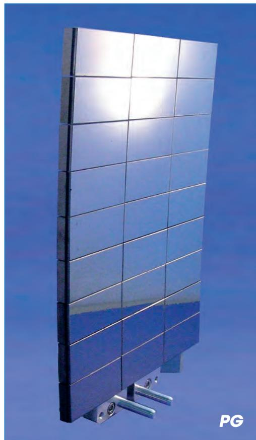
Combined with a  $^3\text{He}$  neutron spin-filter, the aim of the new vertically-focusing Cu(200) monochromator for the **D3** diffractometer will produce a monochromatic beam of polarised neutrons at short wavelengths (0.3 to 0.9 Å). In order to optimise the resolution of the instrument at high take-off angles, several Cu(hhl) planes reflections are accessible when rotating the crystals with respect to the Bragg angle.
