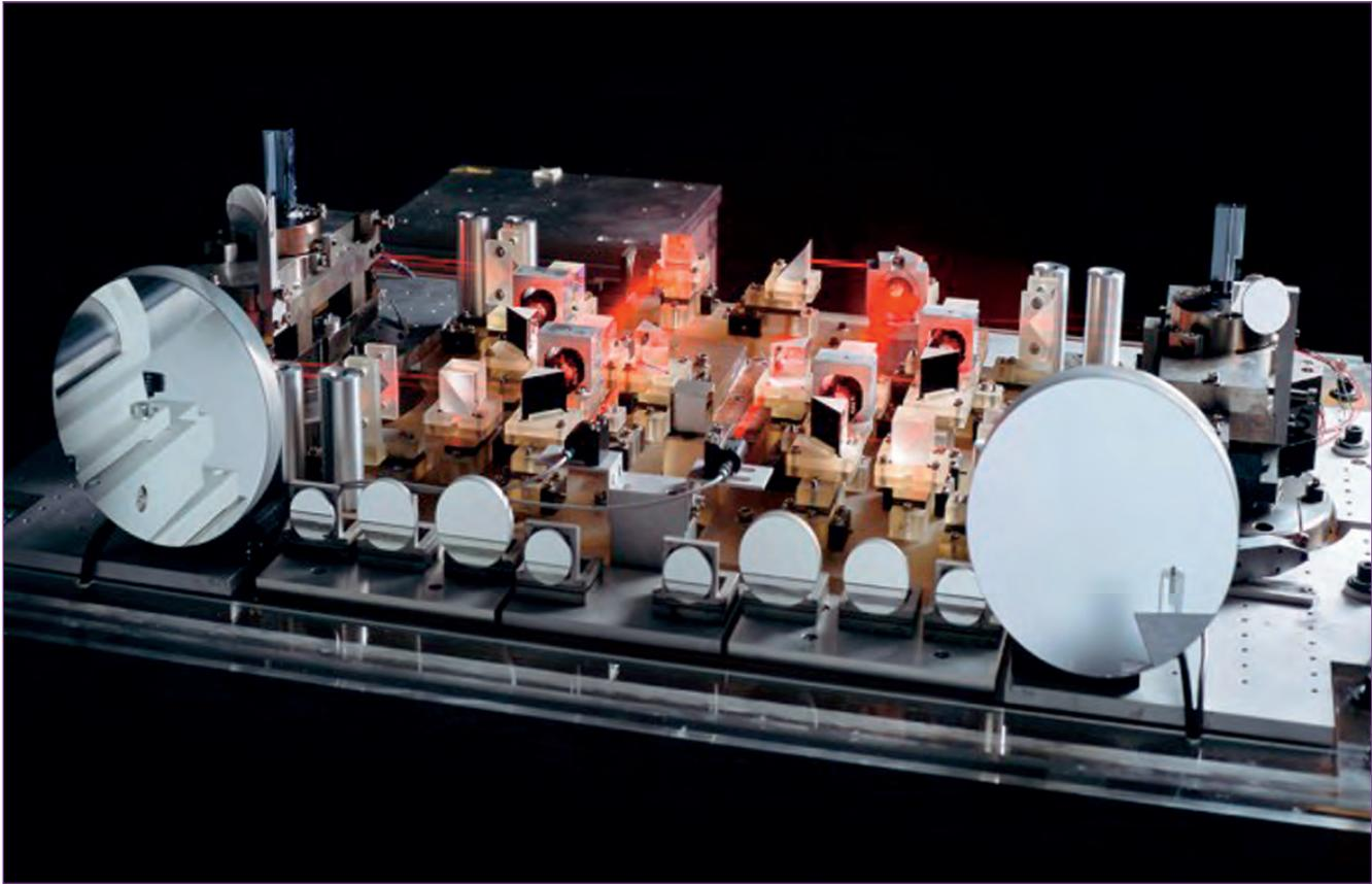
The Gams 5 spectrometer which was used to determine lifetimes and gamma-ray transition energies in the experiment.
