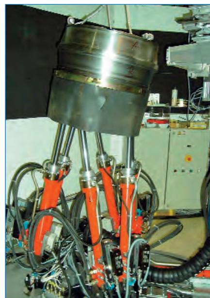
**Figure 3:** Wind turbine and bearing mounted on the SALSAs hexapod.
