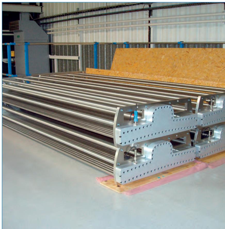
**Figure 3:** Completed detector modules for IN5, each 3 m in length.
