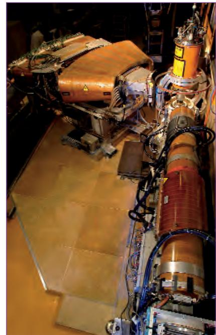
The wide-angle secondary coil/detector of IN11 is essential for the successful investigation of the low-energy magnetic response of frustrated magnets.
