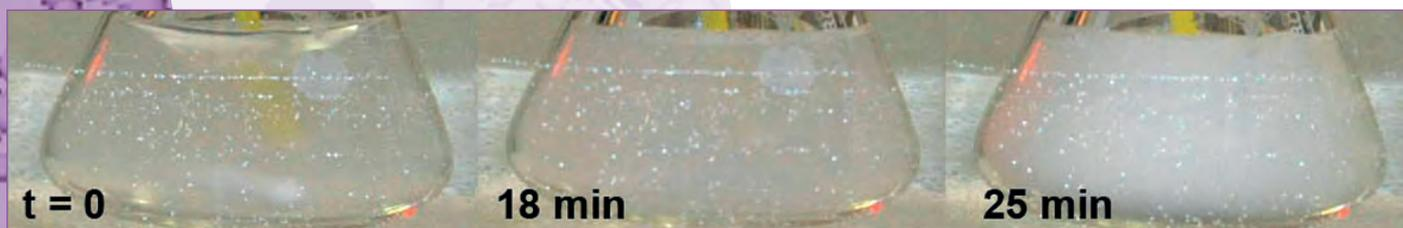
**Figure 1:** Images of the reaction medium at different reaction times taken during the *in situ* SANS experiments. The turbidity of the solution is increasing upon time until a white precipitate forms after 23 minutes.
