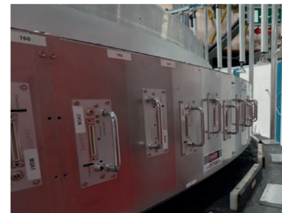
Installation of the new Trench Multi-Wire Proportional Counter (TMWPC) detector on D20c.
