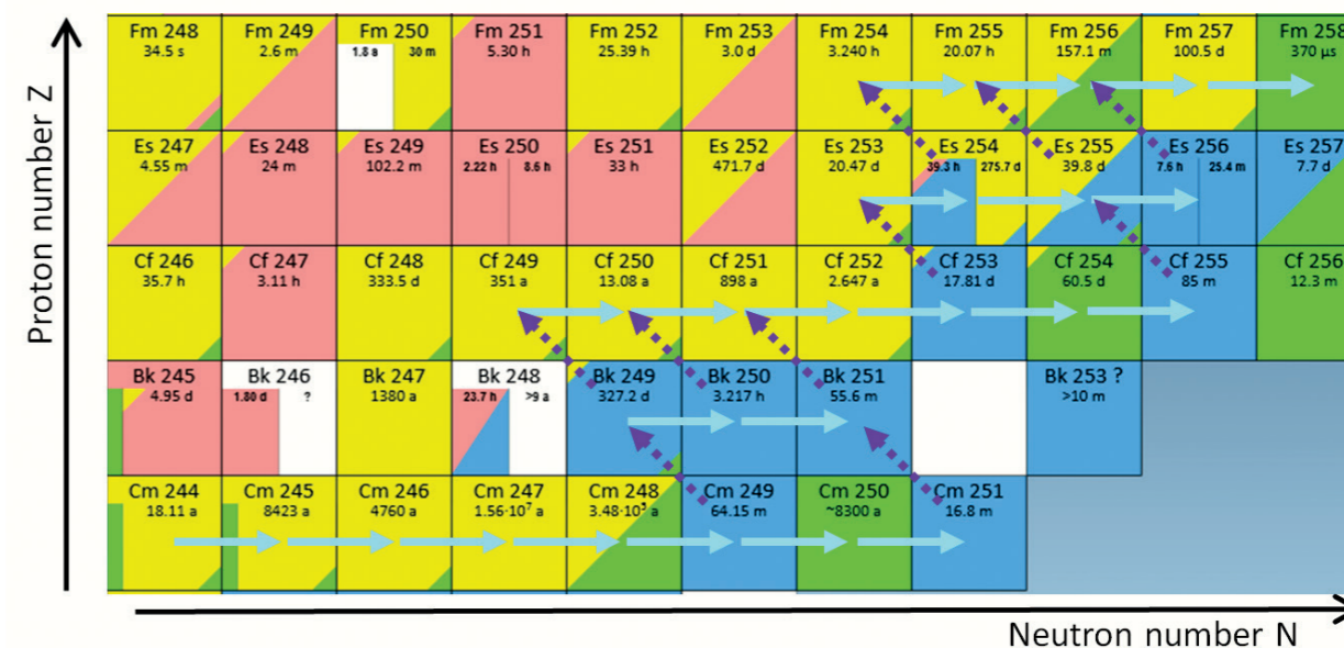
Excerpt from the Karlsruhe Chart of Nuclides. Thermal neutron captures (blue arrows to the right) form heavier isotopes of the same element. Beta-minus decays (violet arrows upwards to the left) transform a neutron into a proton, leading to a nuclide of a heavier element. Combination of both processes can form heavier nuclides of heavier elements. Alpha decays (yellow) and spontaneous fission (green) generate products with lower mass, i.e. are counter-productive to reach heavier masses. Therefore the heaviest element that can be generated by neutron (Z=0) captures is fermium (Z=100).
