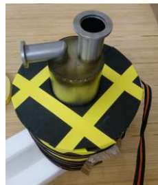
Figure 3.21: 3 He detector surrounded by a boronated rubber shielding (in black on the picture)
