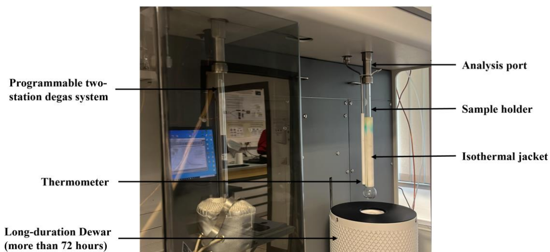
Figure II.7: The ASAP 2020 Instrument from Micromeritics Instruments® at ISTerre, Grenoble.
