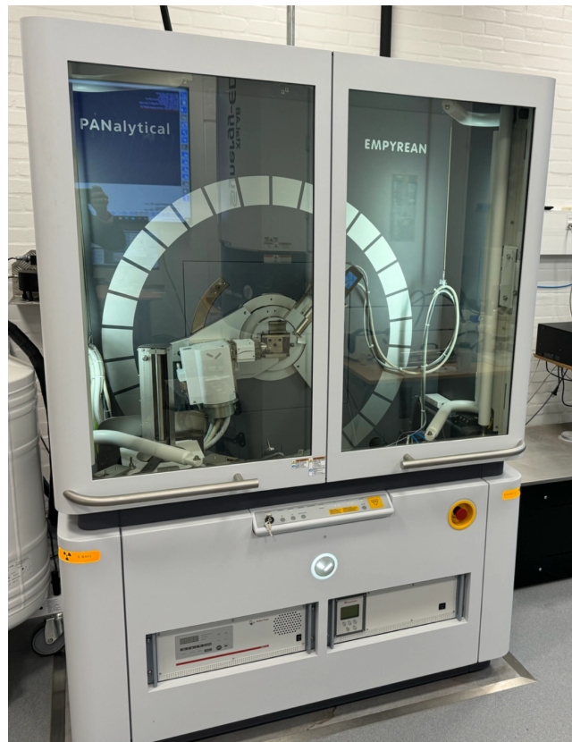
Figure 4.1: Image of the PANalytical Empyrean X-ray diffractometer used for the measurements presented in this work at DTU Chemistry.
