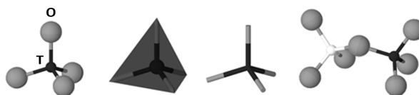
Figure 1.3: Different representations for the basic unit of zeolites, the \text{TO}_4 tetrahedron.
