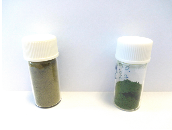
Figure 4.2: Powder samples of (left) \text{LiGaCr}_4\text{O}_8 and (right) \text{LiInCr}_4\text{O}_8 .
