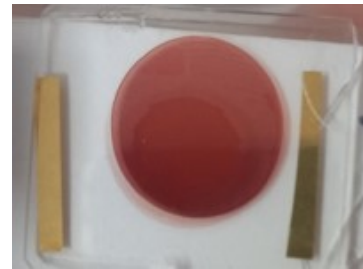
Figure 3.2: NDPC holographic grating recorded in ND-NPC Film
