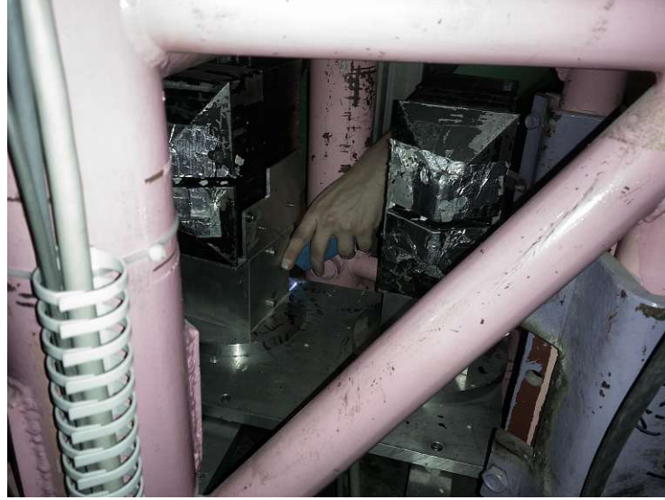
Figure 3.9: Photo of the two magnetic prisms installed at the neutron interferometer station S18 at the Institut Laue-Langevin in Grenoble, France. The adjustment by hand gives an impression of the sizes. The prisms are magnetic yokes with slits at the height of the neutron beam. The magnetic field inside these slits has a field strength of about 1 T. The two spin components of the neutrons traversing the slits are refracted differently, resulting in a divergence between the polarised sub-beams as depicted in Fig. 3.7.
