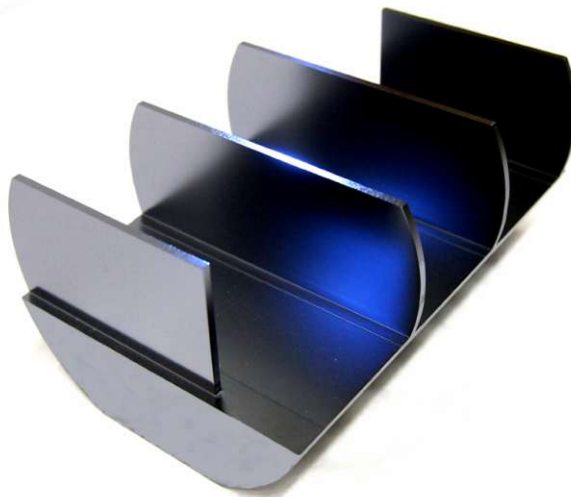
Figure 4.3: Photograph of the four-plate single crystal neutron interferometer used for the experiment presented in this section. The length is about 10 cm. At each interferometer plate, a beam splitting is produced in Laue configuration. This leads to three separated beam paths interfering at the last interferometer plate as depicted schematically in Fig. 4.2.
