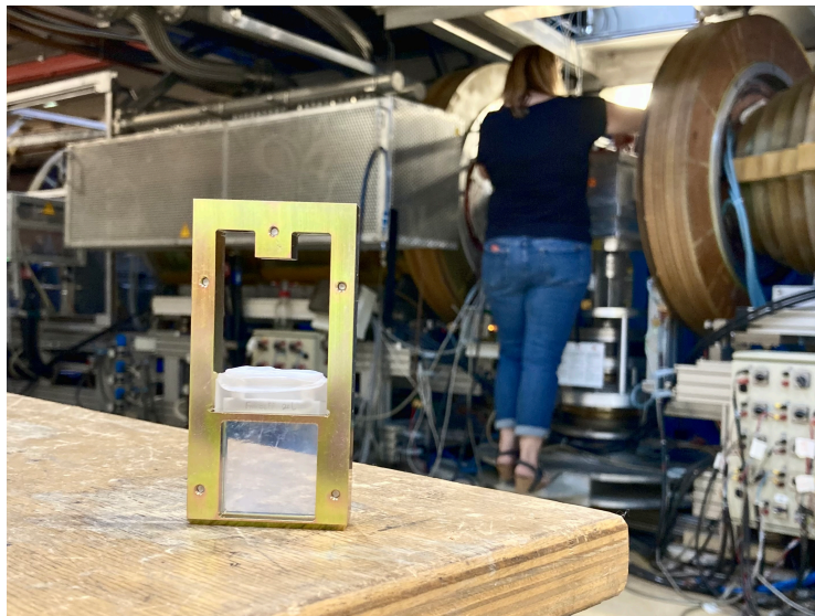
Figure 2.12: Overview of the quartz sample holder containing the FmocFF gel, with the IN15 neutron spin-echo spectrometer at ILL visible in the background.
