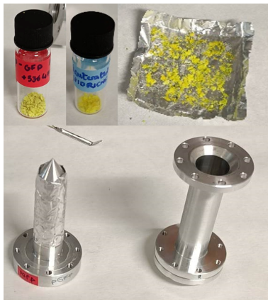
Figure 2-11: Sample preparation for LET, hydrated powder deposited on an aluminium foil wrapped around the inner cylinder of an aluminium hollow cylinder sample holder.
