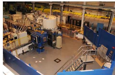
Photo 1: IN16B in its 'low-background' mode, placed in a 'side-of-guide' position analogous to the old IN16.
