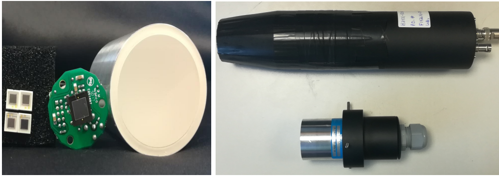
Figure 16: Left: Individual Hamamatsu sensors compared to a \text{LaBr}_3(\text{Ce}) crystal. Right: Size comparison between a PMT tube and the hamamatsu array.
