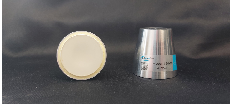
Figure 12: Conical LaBr 3 (Ce) used on the characterization of the SiPM arrays
