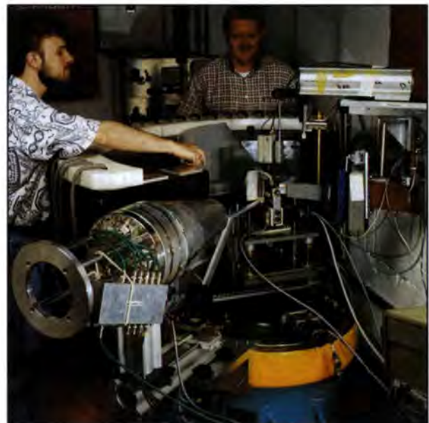
Thilo Pirling (left) and Robert Wimpory show the previous DIA set-up with slits and the position-sensitive detector. The stress rig is on the sample table.
