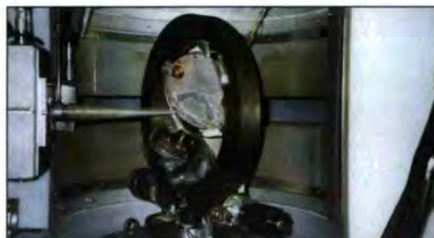
Figure 1b: Disc/disc cell for uniform shear mounted on the Euler cradle of D20. The cell is made from aluminium and has a diameter of 20 cm giving reasonably uniform shear gradients over an area of 1 \text{ cm}^2 near the edge of the cell.
