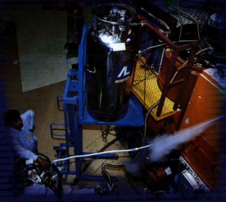
Neville Adroja, Univ. Southampton, fills IN6's cryostat with liquid nitrogen.
