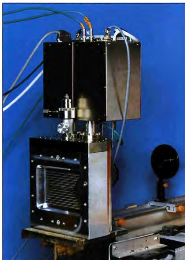
Figure 1: Close-up of the D4C prototype detector (front face).
