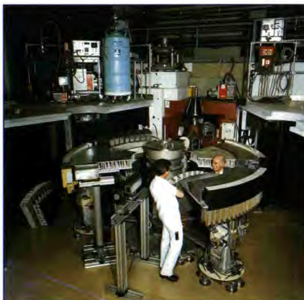
The spectrometer D7 which was used for the measurements reported; René Rebesco (left) and Otto Schärpf are dismantling the guide field.
