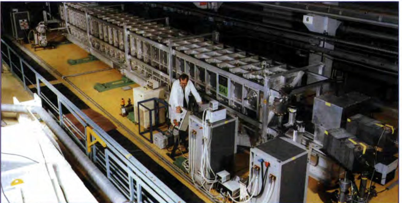
FIGURE 1: Apparatus for measuring h/m_n , installed in the neutron guide hall of the ILL.
