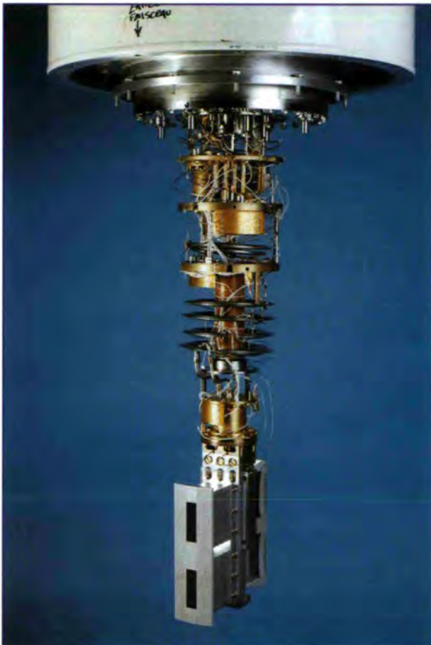
FIGURE 1: Transmission sample cell for ^3\text{He} experiments mounted on the dilution refrigerator. The upper window is used for the ^3\text{He} sample, and the lower for the vanadium calibration sample.
