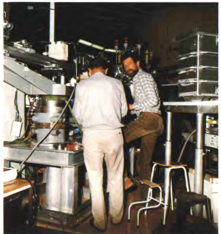
The platform of SN5 is a very busy and rapidly changing experimental area. P. Ageron and W. Mampe (on the right), are two ILL experts in the cold neutron domain. On the extreme right of the picture is a test set-up (collaboration ILL/J.C. Bates; Risley, UK) for a feasibility study of neutron life-time measurements using stored neutrons in bottles with low loss liquid surfaces. On the left is an apparatus for measuring surface reflectivities as a function of neutron wavelengths aiming at the improvement of neutron guides.
