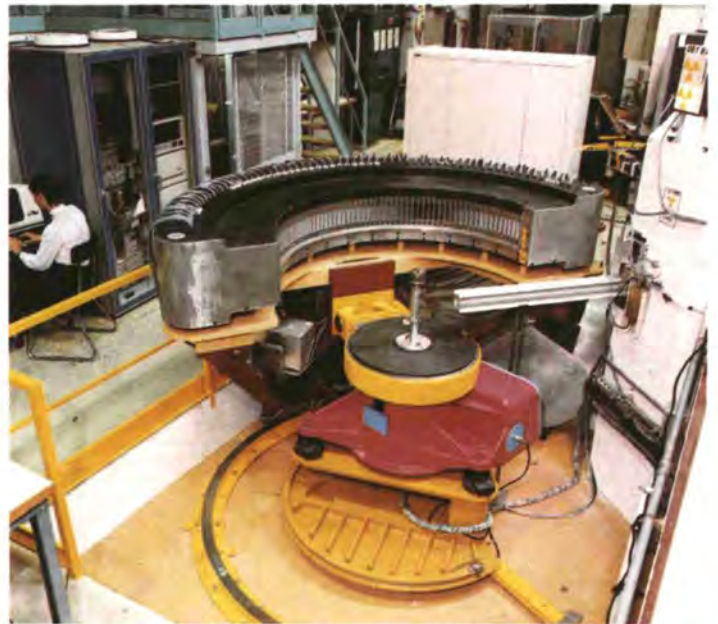
The new D2B diffractometer mounted on its test position at the H22 guide behind D1A/D1B.
