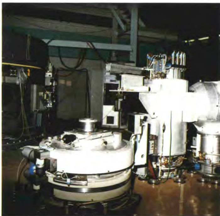
The new IN20 triple-axis spectrometer with polarization analysis and spin-echo option has been moved to its final position on the beam-hole H13. The picture was taken in October 1984.
