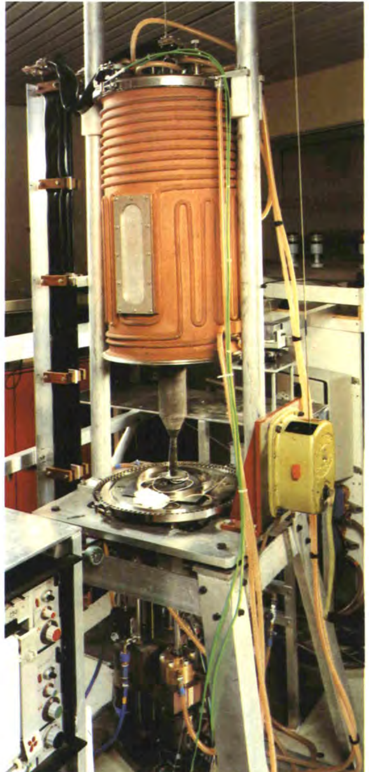
The Bridgman furnace for in-beam controlled growth of large Cu single crystals on the \gamma -ray diffraction facility.
