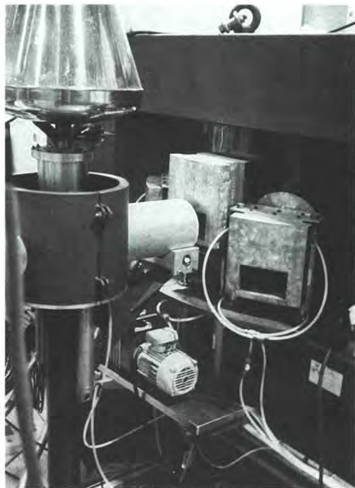
Modification of the monochromator shielding of D7.
