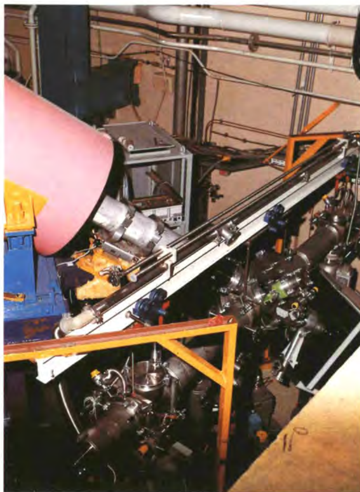
A view of the Cosi Fan Tutte spectrometer before removal (due to the replacement of the inclined beam-tube IH1).
