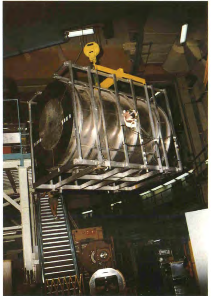
Removal of the storage bottle and shield for the EDM experiment from the platform of SN5 and transfer to the H17 guide.
