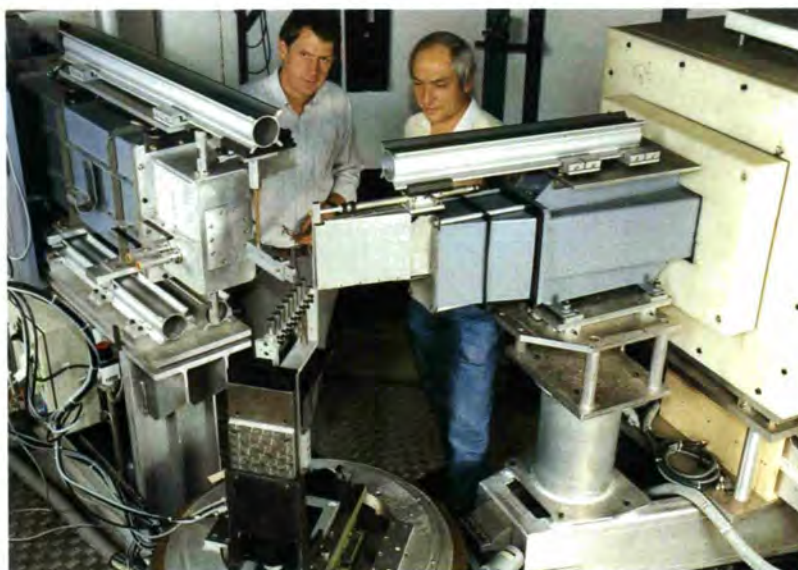
P. Webster (Salford University) (left) and P. Convert at the D20 diffractometer used as neutron strain scanner.
