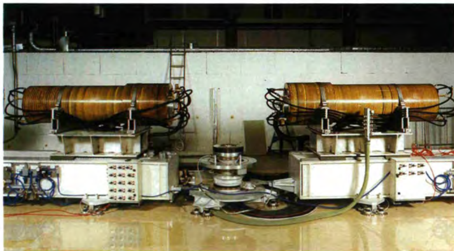
View of the central part of the new Neutron Spin Echo Spectrometer IN15 in the second Guide Hall. In the centre is the sample table with the coils of the guide fields on both sides.
