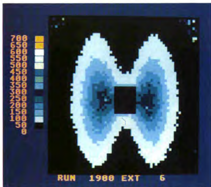
Fig. 55: Trapped deuterated polystyrene chains in a protonated polystyrene network under strain.
