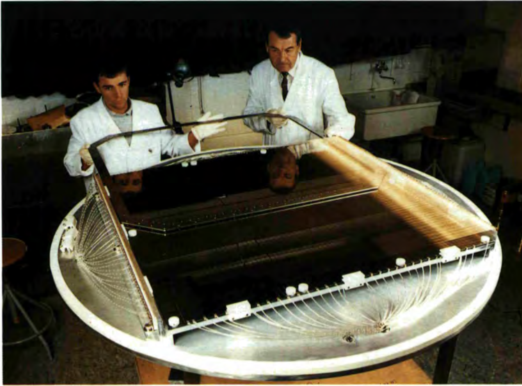
Assembly of the large 64 x 64 - 15 multidetector for HMI-Berlin.
