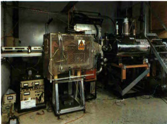
The SUSSEX-NIST experiment on the neutron lifetime, mounted at the beam position SN7. The neutron beam enters from the left. The decay protons are trapped in the cylindrical bottle on the right (superconducting solenoid and electric fields). The high tension part in the middle contains the proton counters.
