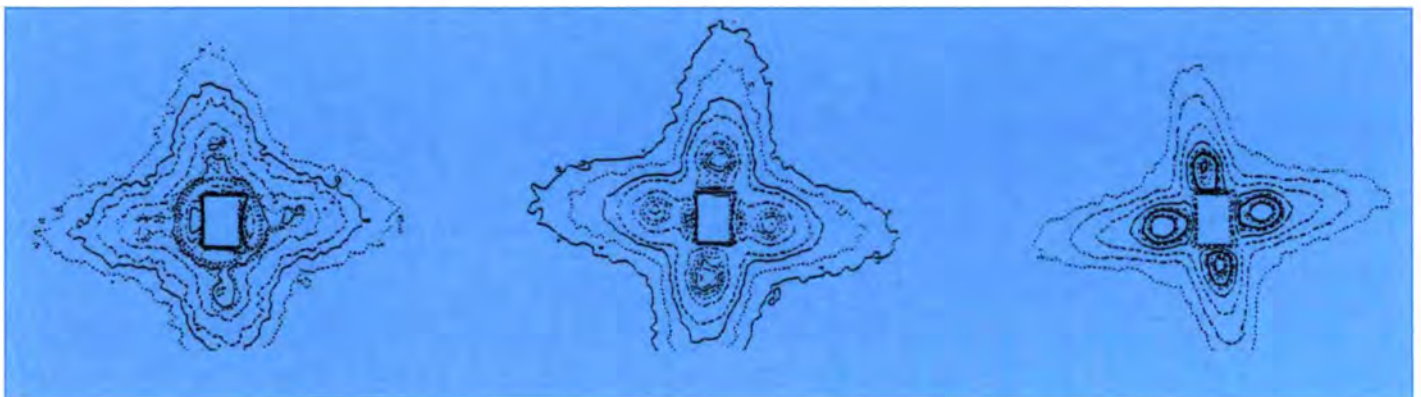
Fig. 38: Iso-intensity map for three samples (from the same single crystal) annealed for: a) 0 hours; b) 2 hours; c) 8 hours on D11, \lambda = 10 \text{ \AA} , D = 35 \text{ m} .
