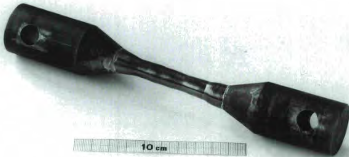
Beryllium single crystal prepared for a tensile experiment.
