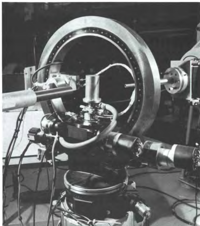
Eulerian sample-orienting cradle on diffractometer D9.
