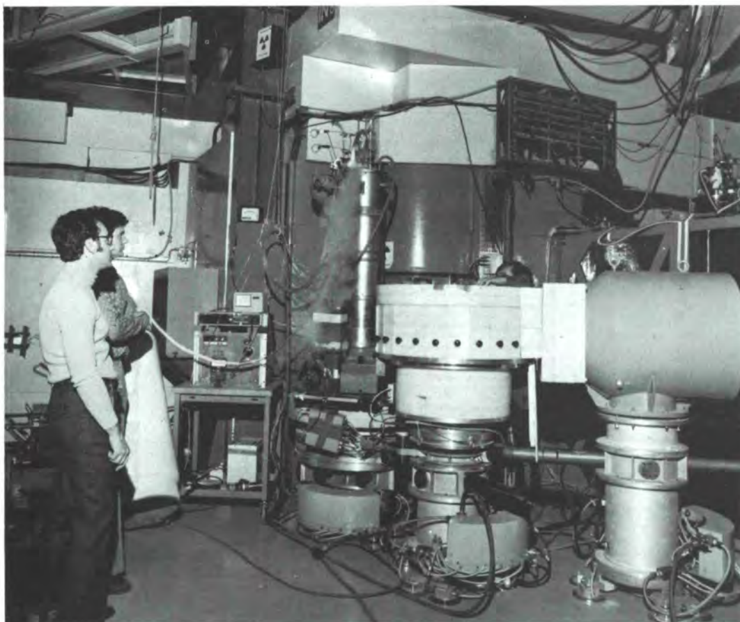
Transferring liquid helium to the cryostat on IN8
