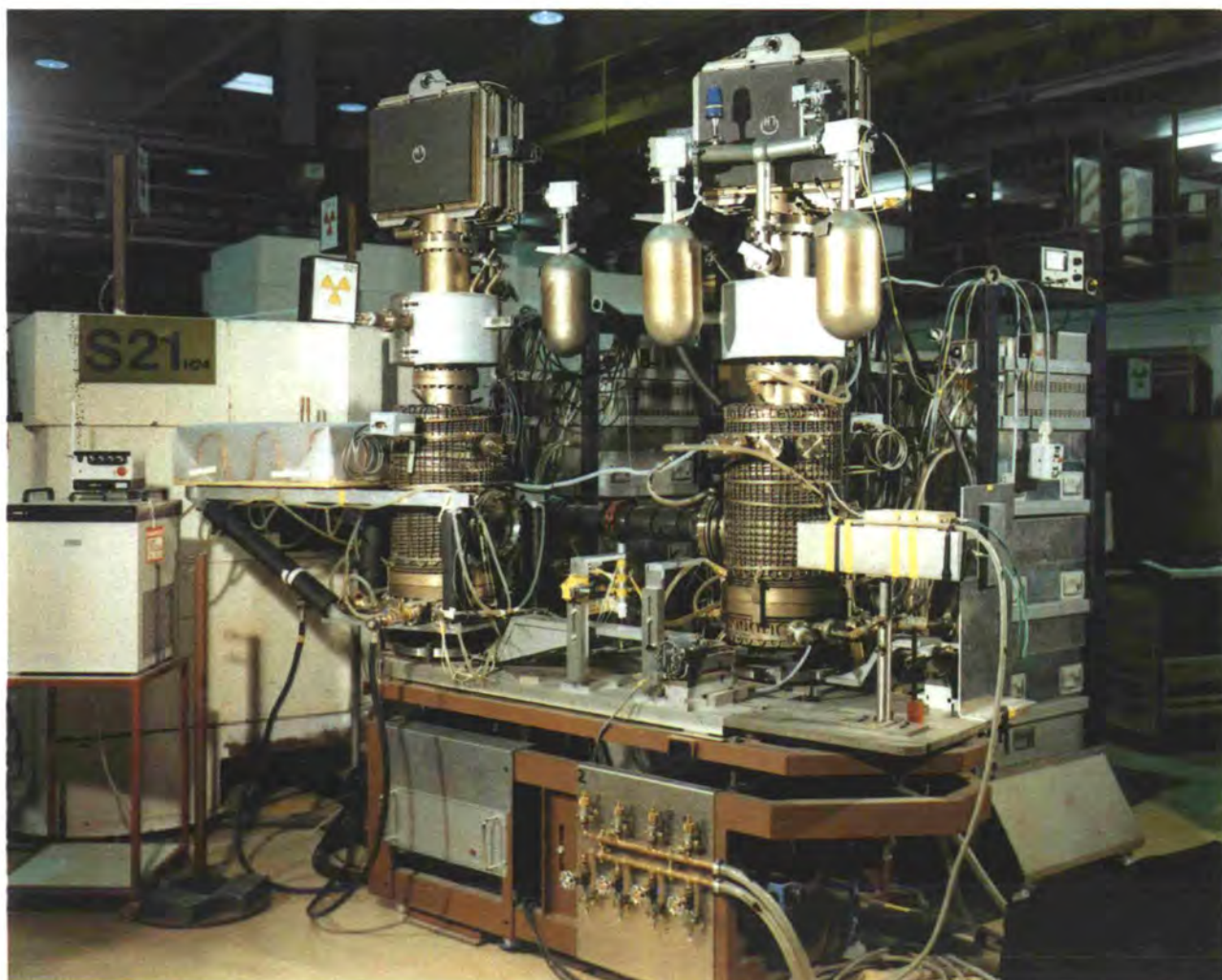
The S21 Double Crystal Diffractometer with high temperature furnaces and laser interferometer.
