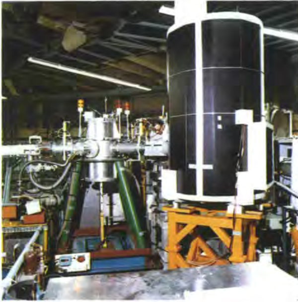
View of the PN5 site. The picture shows the distribution box for providing UCN for the different beam positions (on the left). The UCN microscope can be seen on the right.
