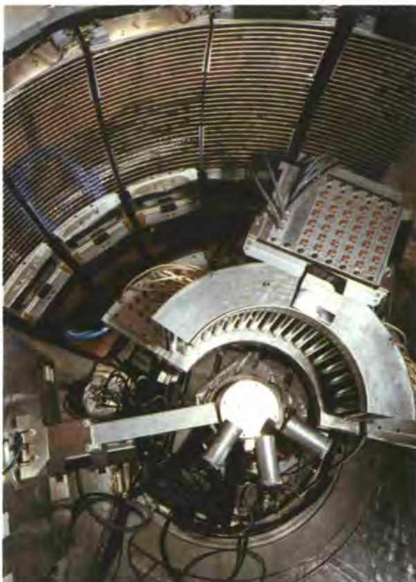
The bank of analyser crystals on the new backscattering spectrometer IN13.
