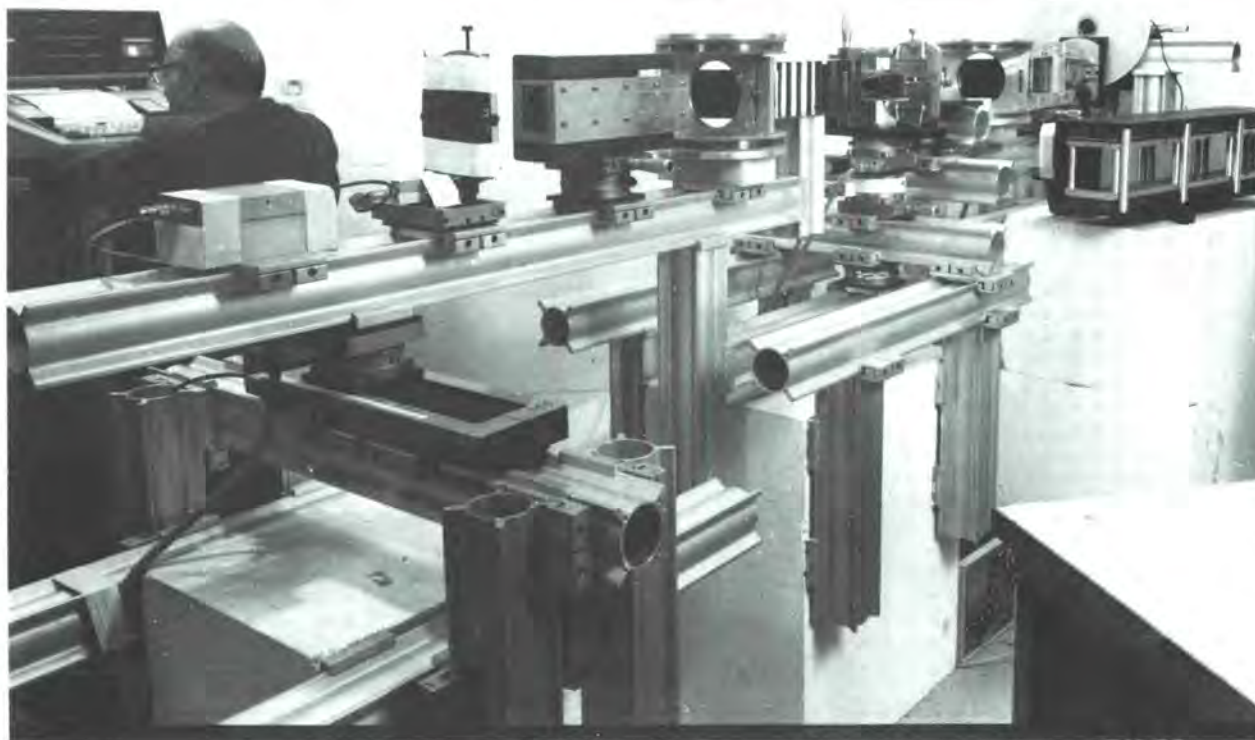
The test facility for super-mirrors and super-benders. On the right is a mounted super-mirror polarizer. On the optical bench (in the middle) a super-bender is acting as analyser.
