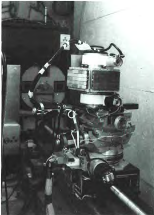
The new vertically curved Cu monochromator set-up on IN8.
