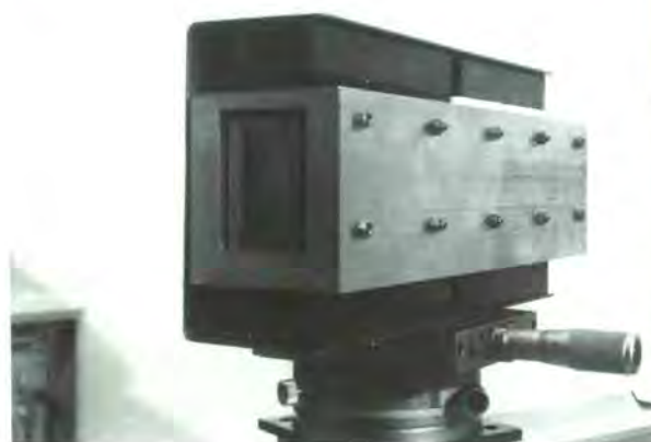
Polariser using curved supermirrors superimposed on an antireflecting layer on very thin glasses (< 0.1. mm) (super-bender).
