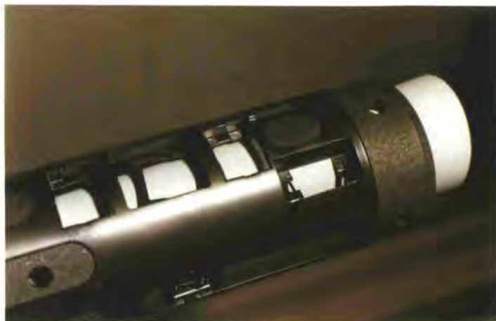
Front part of the new target holder of PN3.
