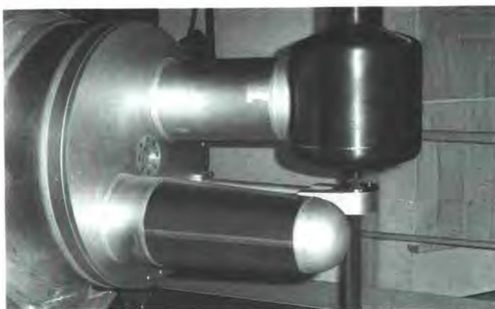
Front view of the H1-H2 in-pile plug for the cold (above) and thermal guides. The new vertical Cold Source can be seen on the right.
