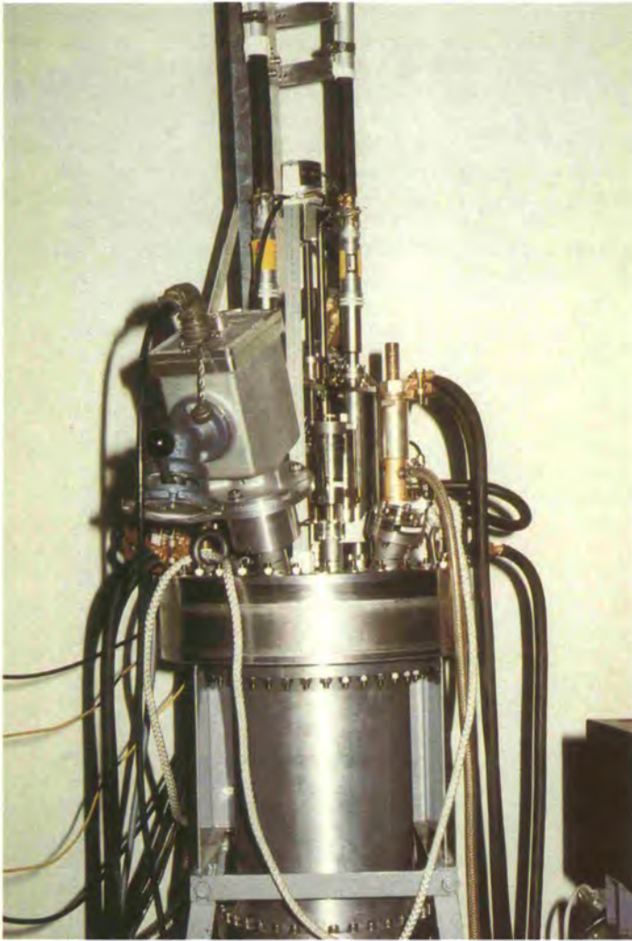
View of the furnace combining crystal growth in situ and neutron scattering experiments.
