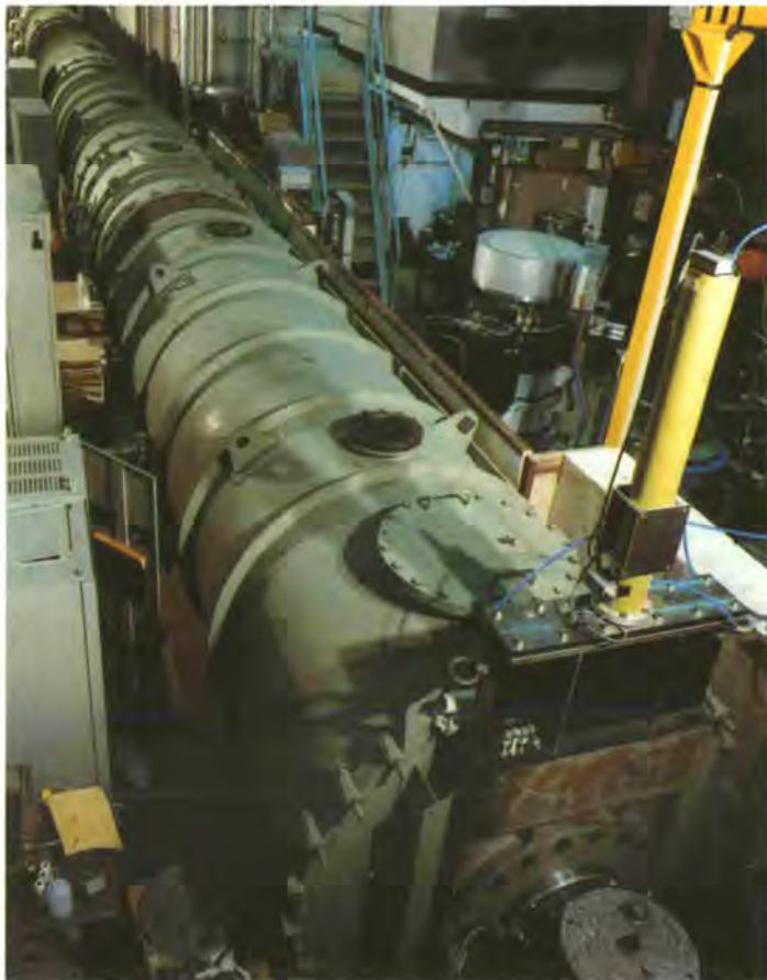
The completed set-up of the new Small Angle Scattering facility D11. The diameter of the flight tube is 1.6 m and the detector may now be placed at any distance from 1 to 37 m from the sample.
