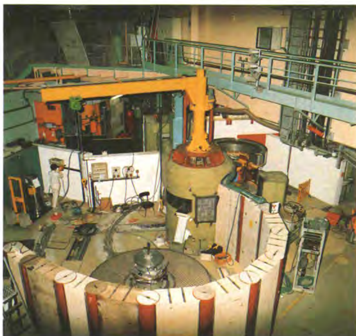
A view of the experimental area around the H11 beam port. The monochromator turret in the middle is feeding 2 instruments: D2B, the very high resolution powder diffractometer (on the right) and D20 a new high flux multidetector diffractometer (in the foreground). A particular feature of the latter is its biological concrete shielding which has been designed such that it requires a minimum of space and yields a maximum of efficiency. The third instrument, the 2D Multidetector D19B is hidden behind the turret.
