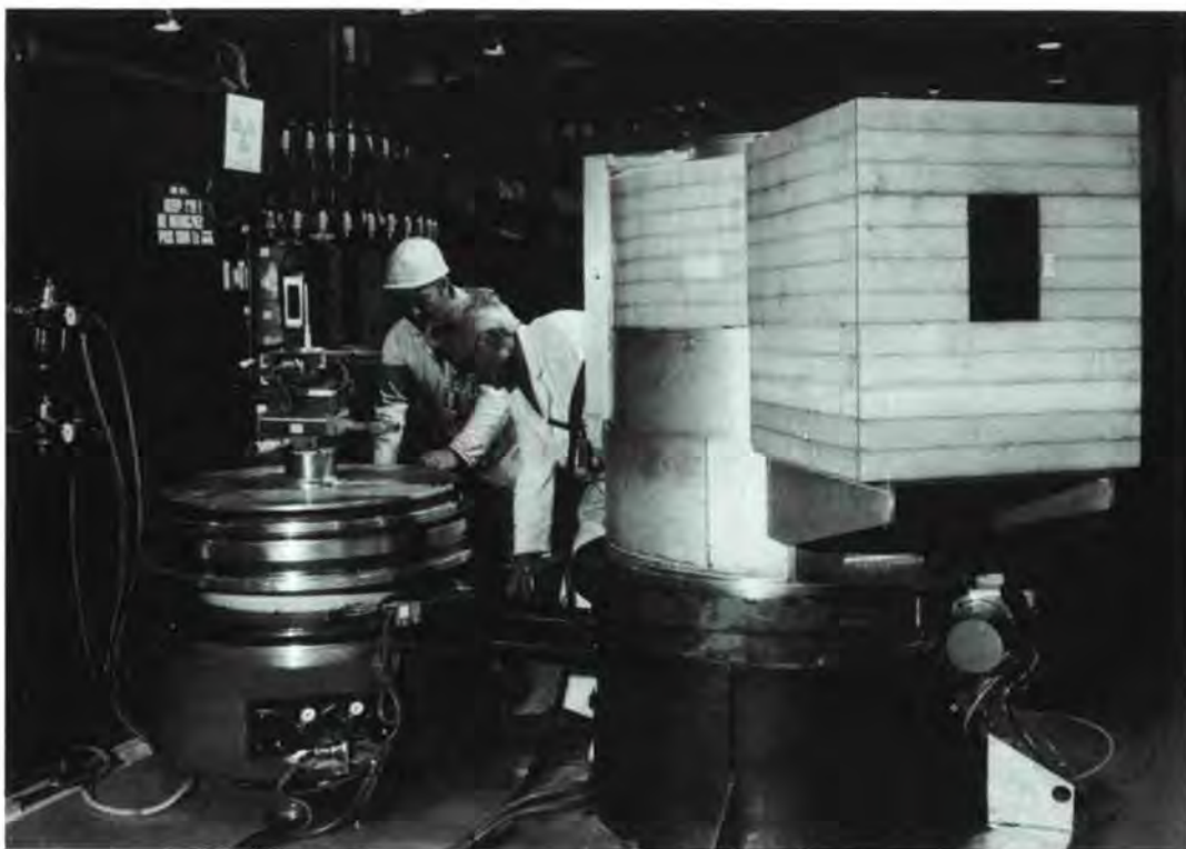
IN12 during construction. On the left is the sample table in front of the monochromator shielding; on the right the analyser-detector assembly.
