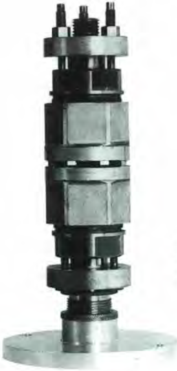
High pressure cell used at ILL for neutron scattering. Maximum pressure is 30 kbar for single crystal samples and 40 kbar for polycrystalline samples. This cell has been designed by the SNCI High Pressure Group.
