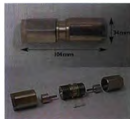
Figure 1: Photographs of the 30 kbar non-magnetic clamp cell designed at the Institute for High Pressure Physics and used in the 10T cryomagnet on the polarised neutron diffractometer D3.
