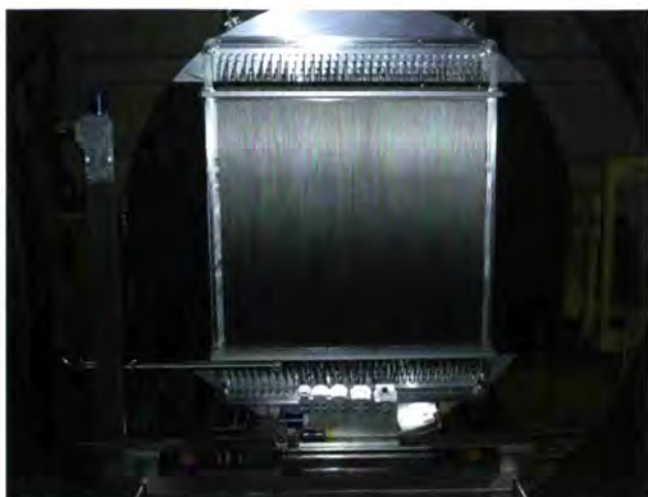
The fast small-angle detector on D22.
