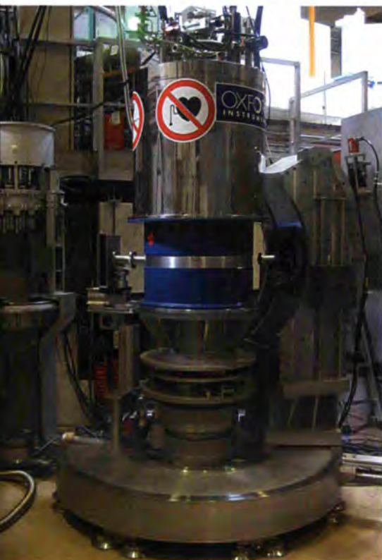
Figure 1: The new D23 secondary spectrometer with the 15 T ILL cryomagnet mounted.
