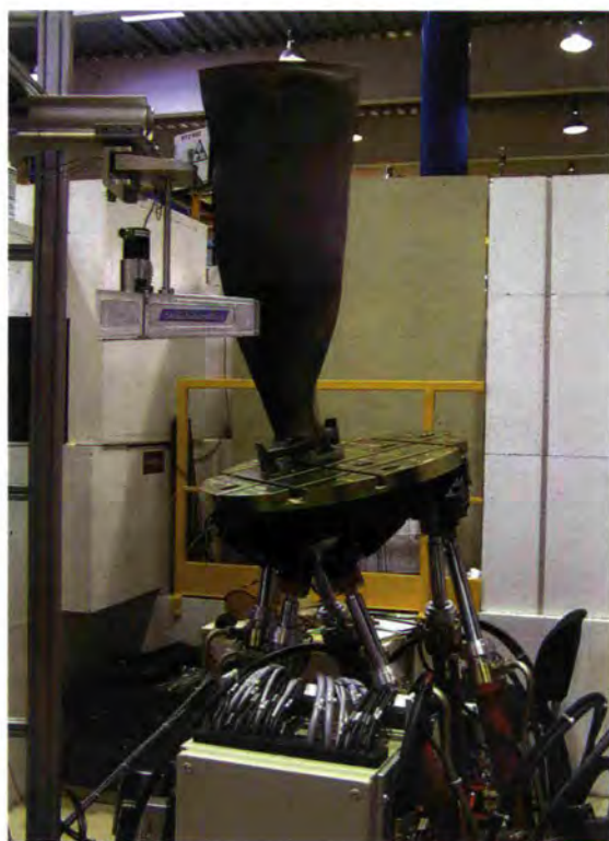
A Fan-blade of an aero-engine (about 1 m high) mounted on the hexapod sample stage of SALSA . On the left: the automated variable slit system for beam definition.
