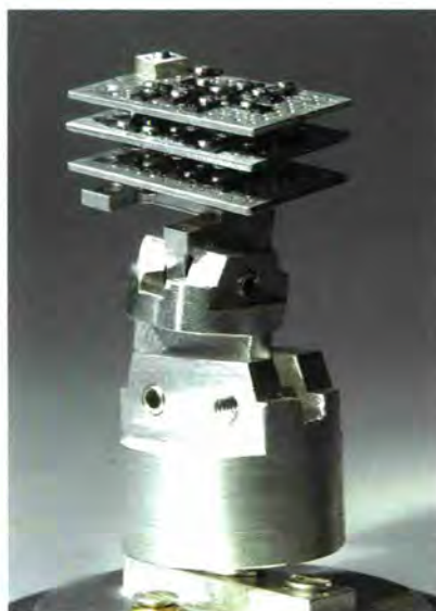
Figure 1: A sample plate showing that crystals are fixed by Al-screws to avoid incoherent hydrogen scattering from organic glue. The complete assembly is shown below.
