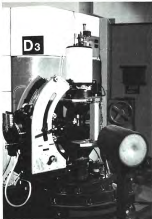
The new polarised neutron two-axis diffractometer D3.
