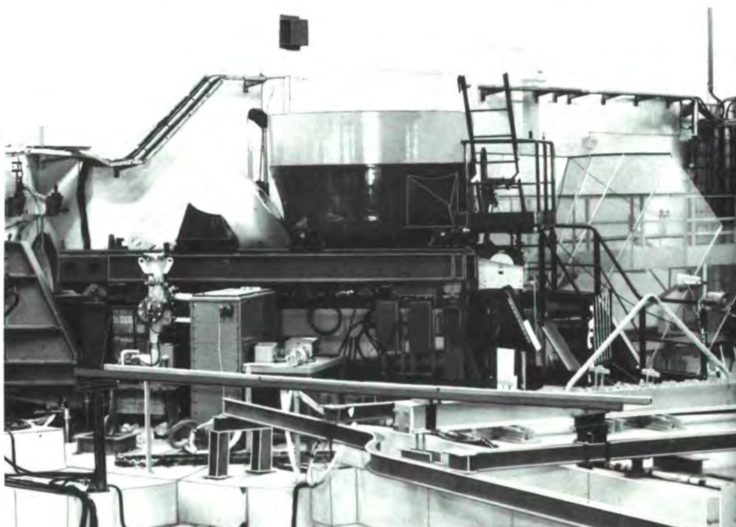
The new four-circle Mark VI diffractometer D15 on the inclined hole IH4
