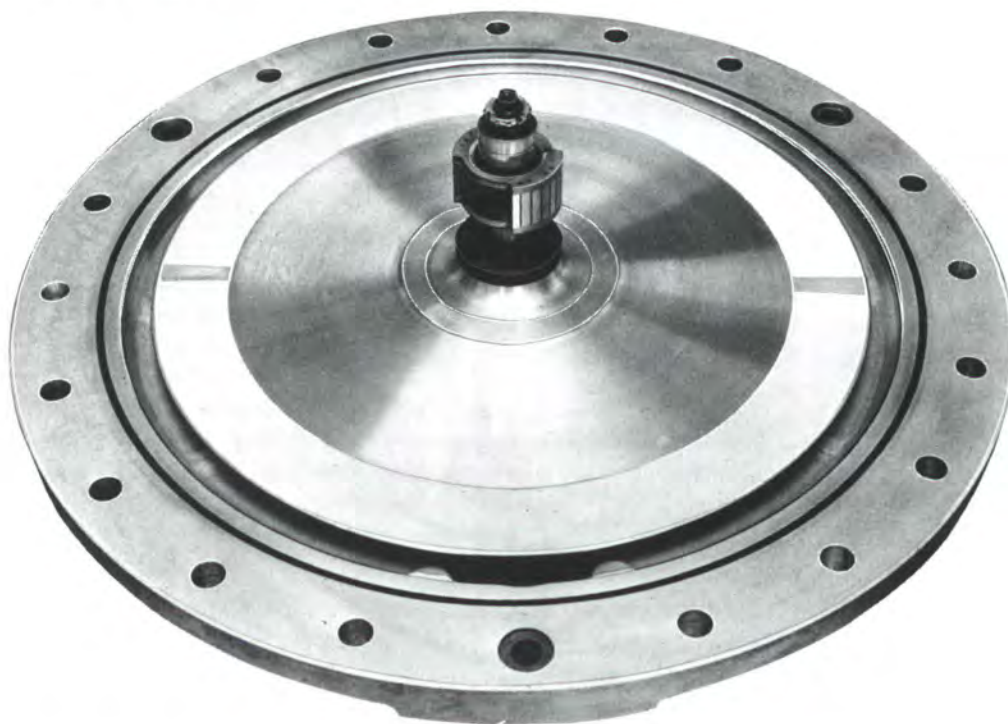
Chopper disk for the multi-chopper spectrometer IN5.
