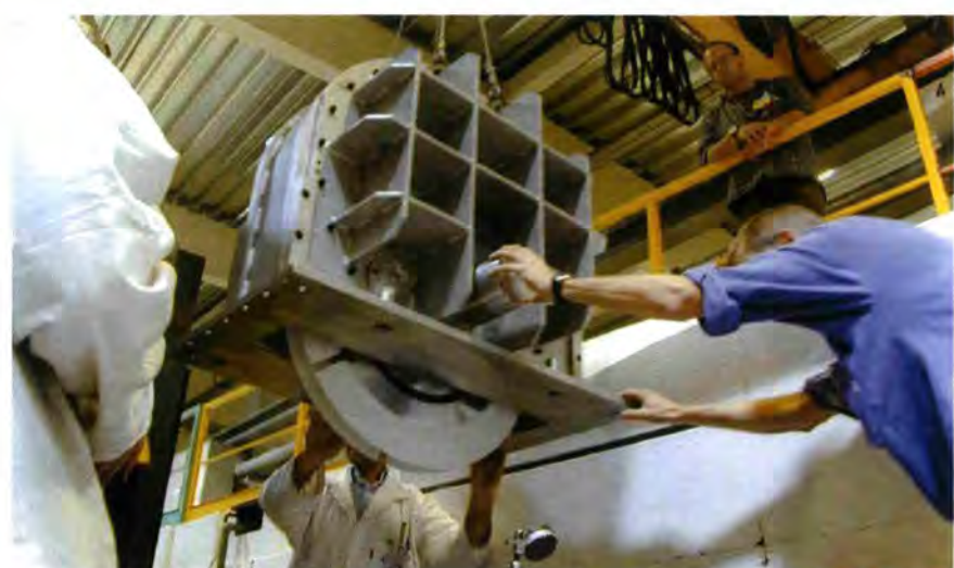
Figure 1: Installation of one of the IN5 double choppers: with very small gaps between chopper disks and guides - this is precision work.
