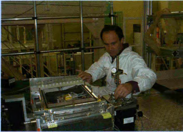
The set-up used by Valery Nesvizhevsky and his team for the detection of quantised states of neutrons in the gravitational field of the earth.
