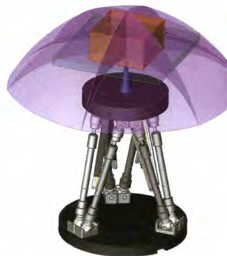
Figure 2: Stewart platform showing two possible work volumes, within the complex and total volume available. (Courtesy of William Hutt, Manchester University-ILL)
