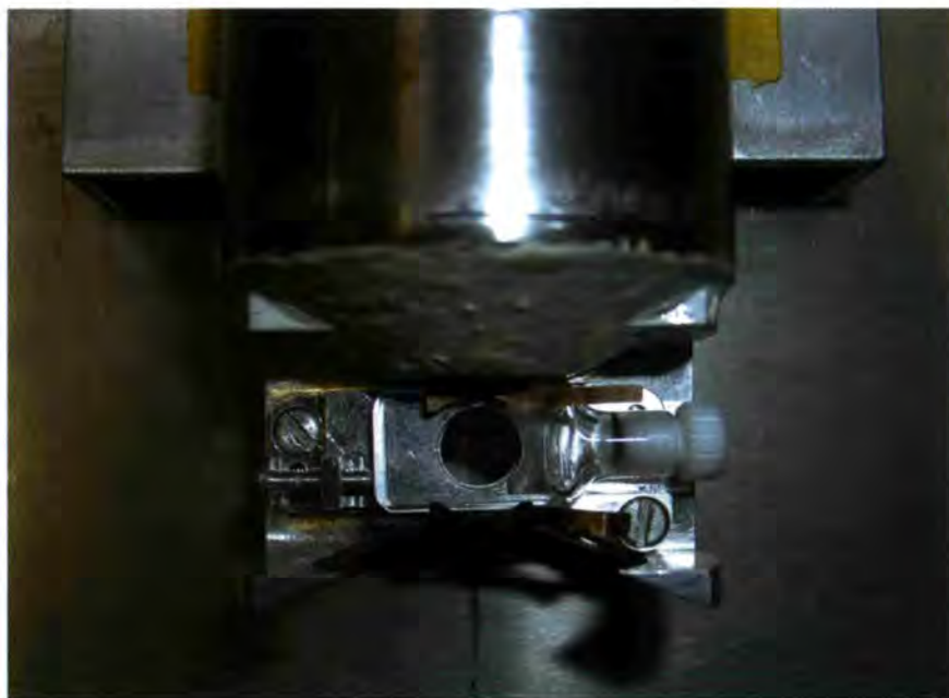
New magnet sample holder for SANS experiments under vacuum at D11, developed at ILL for AEA Technology. The photo shows a 1mm standard water cell at the sample position. The sample holder is shown before fixation to the upper magnet pole piece, the lower pole piece is not shown.
