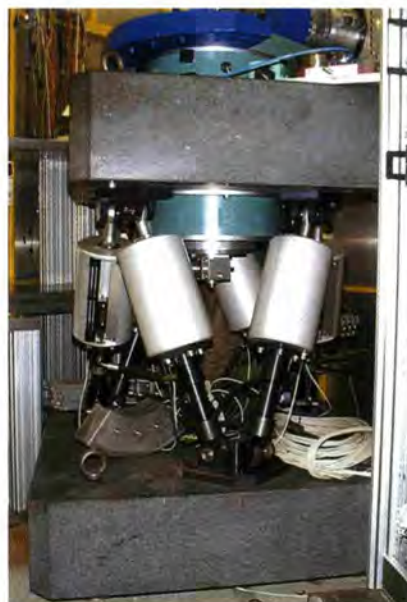
Figure 1: Stewart platform with a repeatability in X, Y and Z better than 5\mu\text{m} , and a load capacity of 20 kN. (Courtesy of European Molecular Biology Laboratories, Hamburg)
