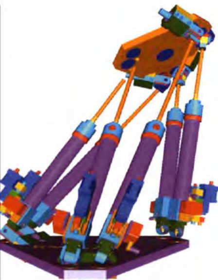
Figure 4: CAD 3D image of the proposed Stewart platform being developed for the ILL. (Courtesy of OHE)
