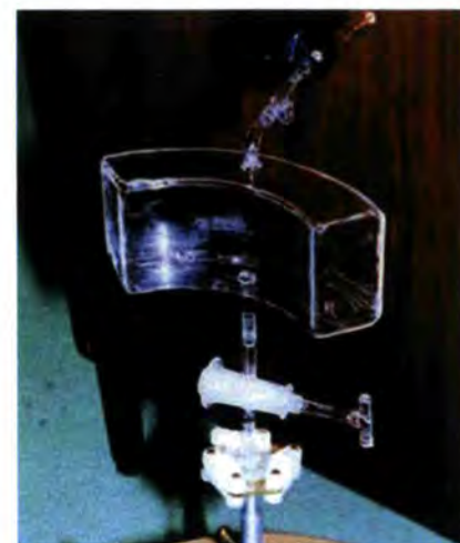
Figure2: The ^3\text{He} spin filter used in this measurement, produced at the ILL by W. Heil and H. Humblot. The horizontal coverage of the cell is 90^\circ , and the height of the cell is 70 mm. The cell contained 2.7 bar of ^3\text{He} during the measurement.
