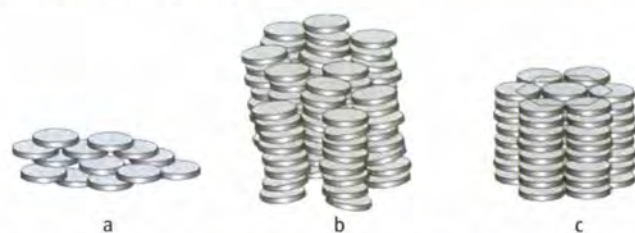
Figure 1: Liquid crystalline phases with increasing molecular order. In order of decreasing temperature: a) Nematic discotic, b) nematic columnar, c) columnar hexagonal.
