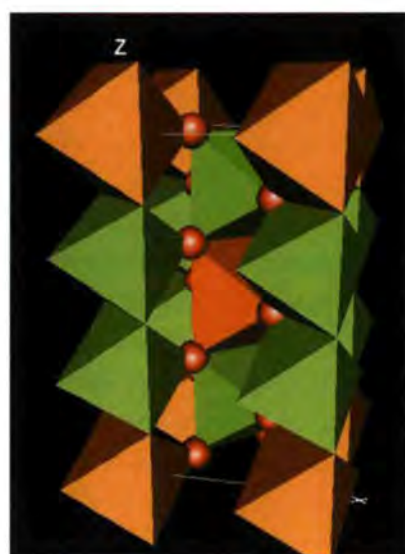
Figure 1: Schematic of the \text{FeTa}_2\text{O}_6 structure. Fe and Ta are both octahedrally coordinated to O atoms at the vertices of the volumes shown. Fe is in the centre of each brown octahedron, Ta in the centre of each green.
