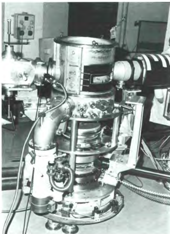
The new liquids diffractometer D4 B at the Hot Source which will become routinely available to users in Summer 1983.
