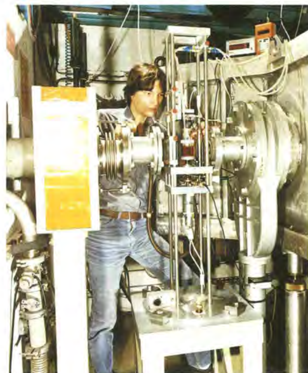
Adjusting the temperature and speed controlled shear gradient apparatus for liquid samples at the sample position A of D11. The sample to be investigated, a dilute V_2O_5 solution of deep red colour in water, is contained in the 0.5 mm gap between the adjustable (fixed) inner piston and the outer (rotating) cylinder, both ground from quartz glass which is transparent for neutrons.
