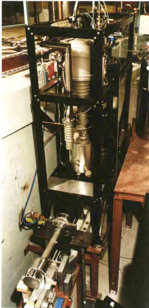
The new superthermal UCN source installed at H 17. The lower part shows the 3 m long He container in which UCN are produced. The vertical section houses the various cooling circuits.
