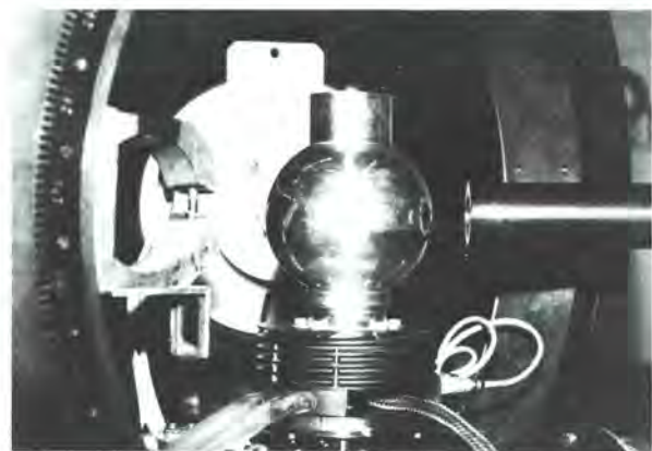
New four-circle furnace (constructed at Kernforschungszentrum Karlsruhe) in operation on D9.
