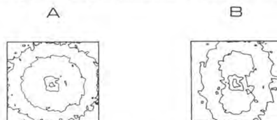
Fig. 4: Scattering from colloidal V 2 O 5 in D 2 O (12.5 mg/cm 3 ) on the two-dimensional detector of D11.
