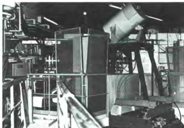
PN 8, the new coincidence fission spectrometer "Cosi fan tutte", installed on the inclined hole IH1.
