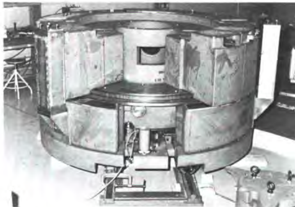
The assembling of IN 20 in the test hall. The picture shows the monochromator drum of the instrument.
