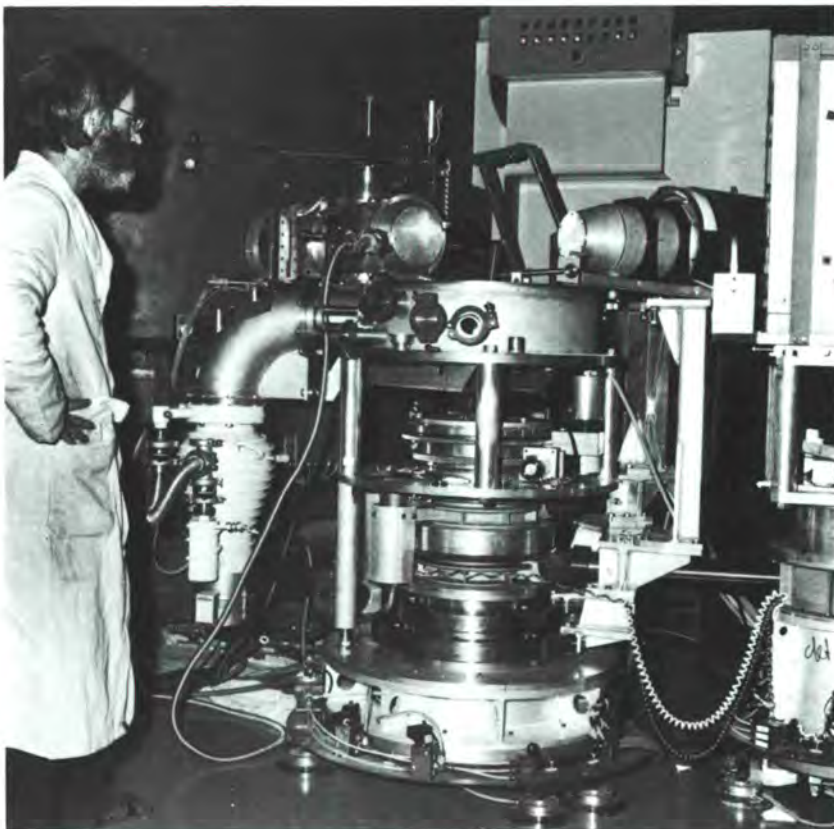
The new liquids diffractometer D4B is presently being tested and will be available to users as from Summer 1983
