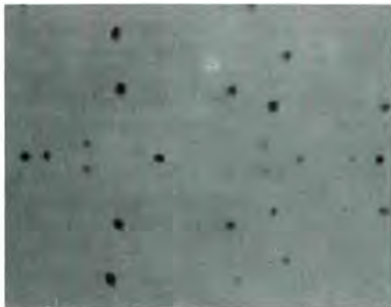
Fig. ii. - A 6° oscillation photograph of DyMn 0.4 on D12 at 20K (exposure time 30 minutes).
