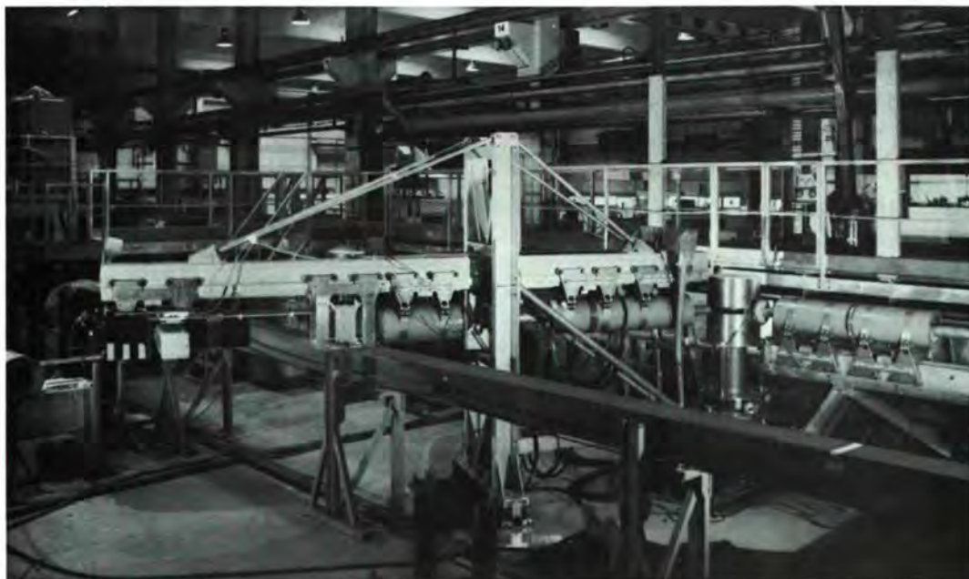
The IN11 spin-echo spectrometer operating at 80^\circ scattering angle. The incident beam is raised by a vertically S-bent guide to allow clearance of the D11 collimation system.
