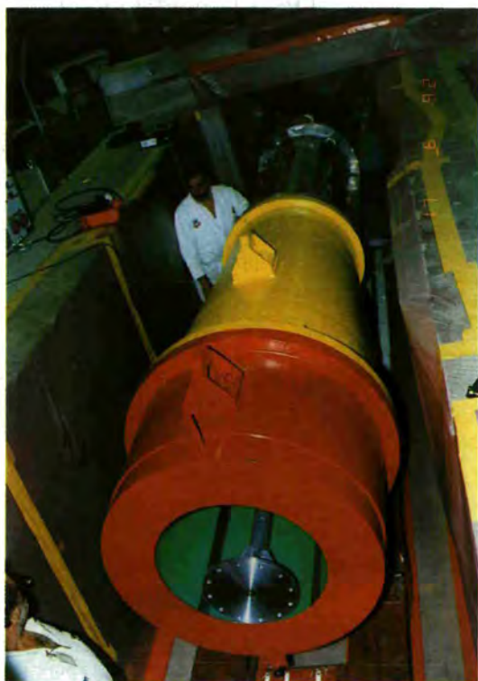
Lead coffin for the removal of the H5 liner (Horizontal Cold Source).
