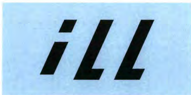
Fig. 4a: Letters of the ILL-logo "iLL" made from neutron absorbing B_4C . The distance between point and line of the "i" is 2 mm.
