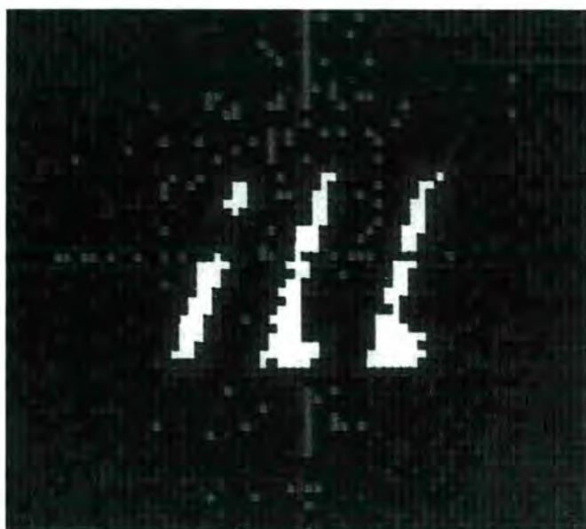
Fig. 4b: Neutron image of the above letters taken with a microstrip gas detector. Since reactor neutrons are presently not available, the detector was irradiated by a collimated Am-Be source. The exposure time was 240 hours at a rate of 4 counts per second. (see also picture on page 2).
