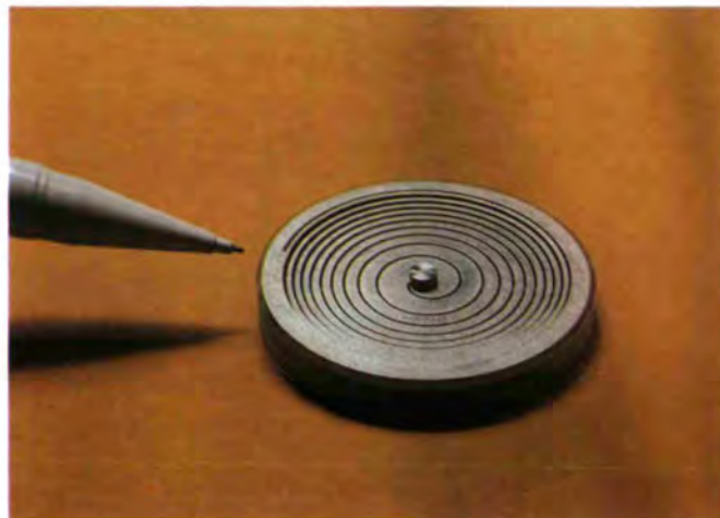
Double-spiral correction coil to be used on IN20 TASSE as part of the design of the new superconducting OFS precession coils (see report "Instrument Groups", 3-axis spectrometers).
