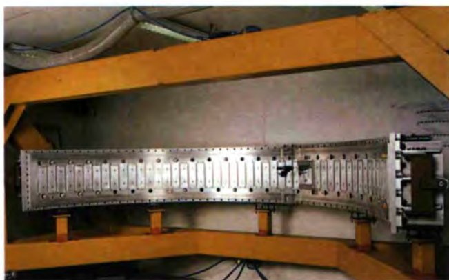
The new multidetector for the high flux diffractometer D20 (see report on page 124).
