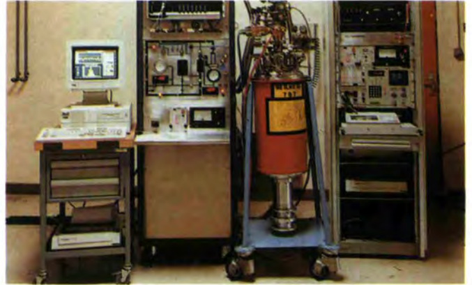
Automation of the dilution refrigerator inserts (see report on page 104).
