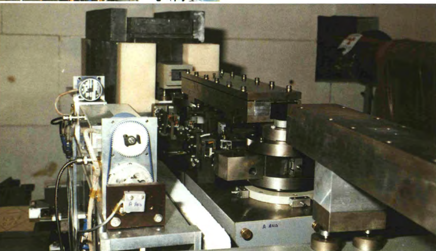
The double flat-crystal \gamma -ray spectrometer (GAMS 4) installed at the H6-H7 beam-tube by a team from the NBS Washington.
