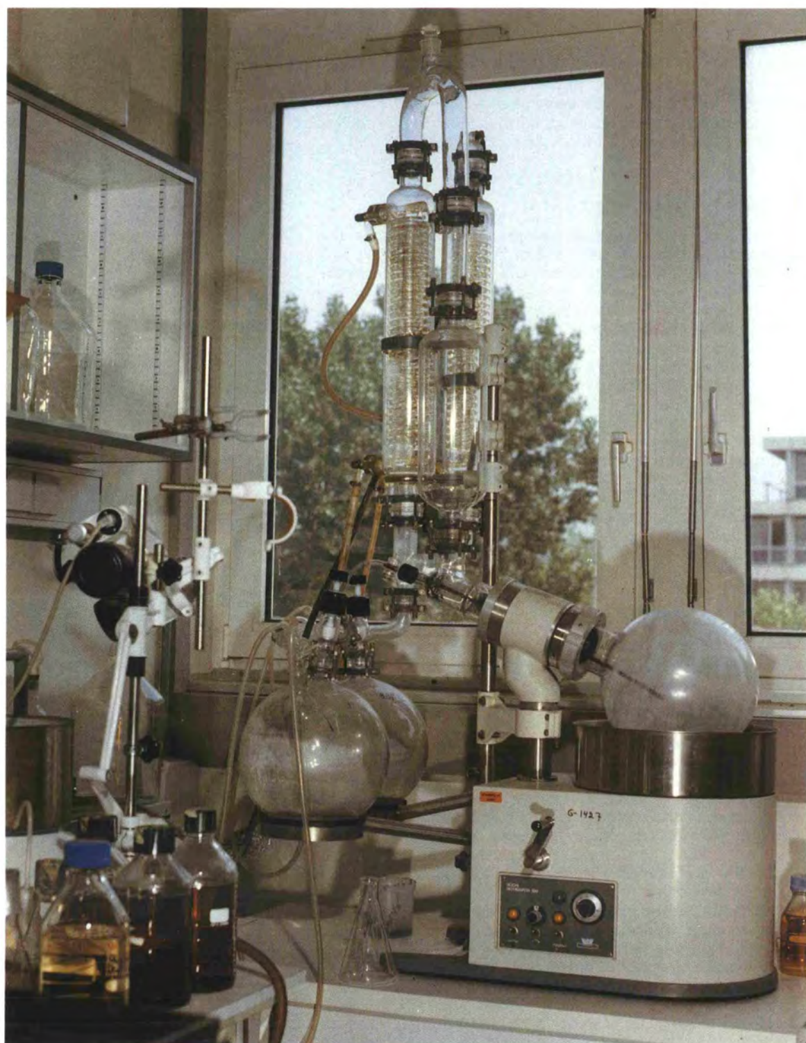
Laboratory equipment of EMBL: Recovery of ^2\text{H}_2\text{O} from fermentation process by vacuum distillation.
