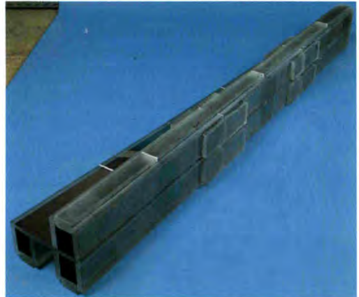
Shunt of neutron guides for the second cold source
