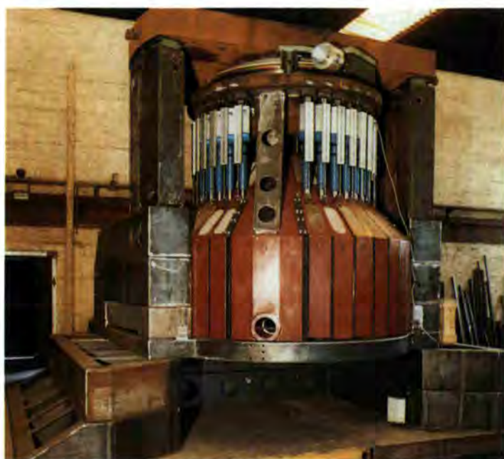
Monochromator drum for IN14, the new 3-axis spectrometer on the second cold source.
