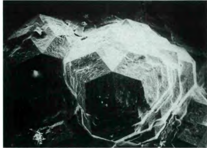
Figure 36: Millimeter size grain which is a single quasicrystal of Al_6Li_3Cu (courtesy of Pechiney, Centre de Recherche, Voreppe)
