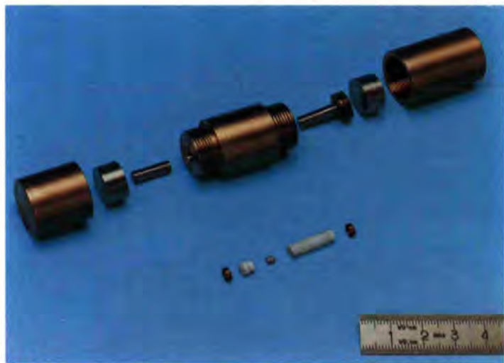
High pressure BeCu cell for studies under magnetic fields.
