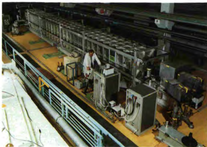
S50: It is the aim of S50 to determine h/m ( h : Planck constant, m : neutron mass) to an uncertainty of 10^{-6} . As h/m = \lambda/v , one has to measure the wavelength and the velocity of the same neutrons. In S50, a beam of neutrons of well-known wavelength is produced by back-reflection on a perfect Si-crystal. The velocity is measured by a refined time-of-flight method (using polarized neutrons, phase modulation and interference patterns). The photograph shows the vacuum vessel of about 20 m length containing the experimental equipment for the determination of h/m .
