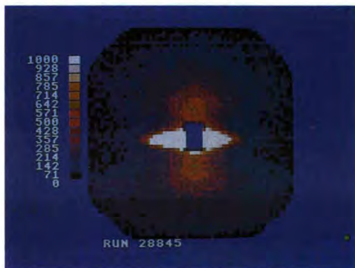
Figure 76: SANS from concentration fluctuations in a mixture of Polystyrene and Poly(phenylene oxide), deformed below T_g (stretching direction horizontal).
