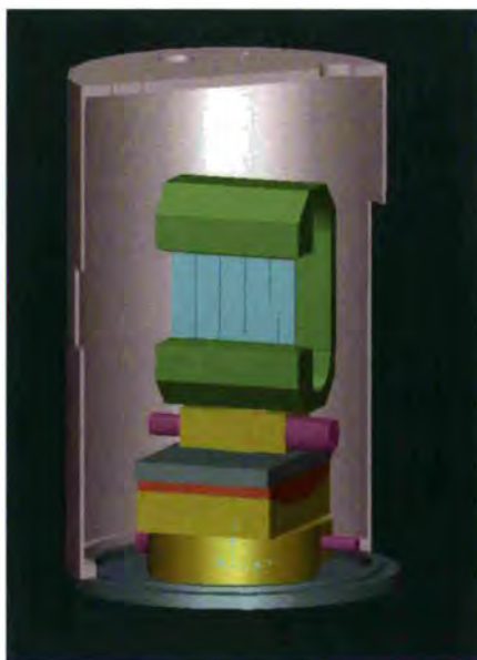
Schematic drawing of the new IN20 monochromator assembly, the biggest one ever built (230x150 mm 2 , composed of 75 crystals).
