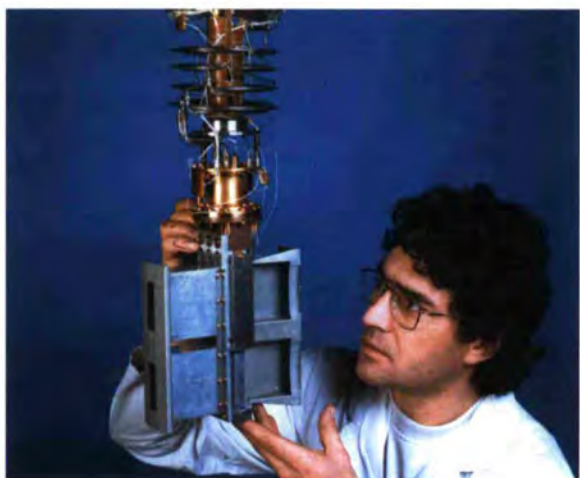
Jean Paul Gonzales checks the inside of the 6mK dilution refrigerator.
