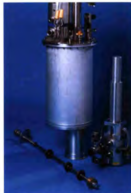
Figure 2: Picture of the ILL top-loading cryocooler (left) and of the XMAS bottom-loading cryocooler (right). In foreground, the sample-holder of the top-loading machine (length 910 mm).
