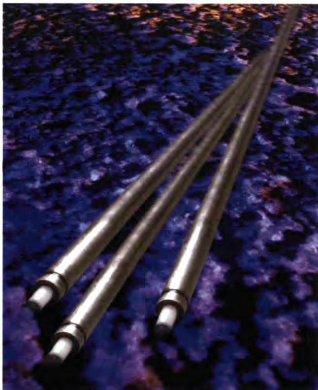
Prototypes of the D22 tubular position sensitive detectors (length of the tube: 1m)
