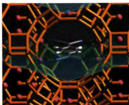
Figure 2: TCNQ in the 12-ring window of the NaY and HY framework; Na=pink, C=grey, H=white, N=blue; (200)-plane=blue.
