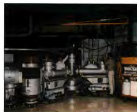
Figure 1: The three-axis spin-echo (TASSE) precession coils mounted on IN20.
