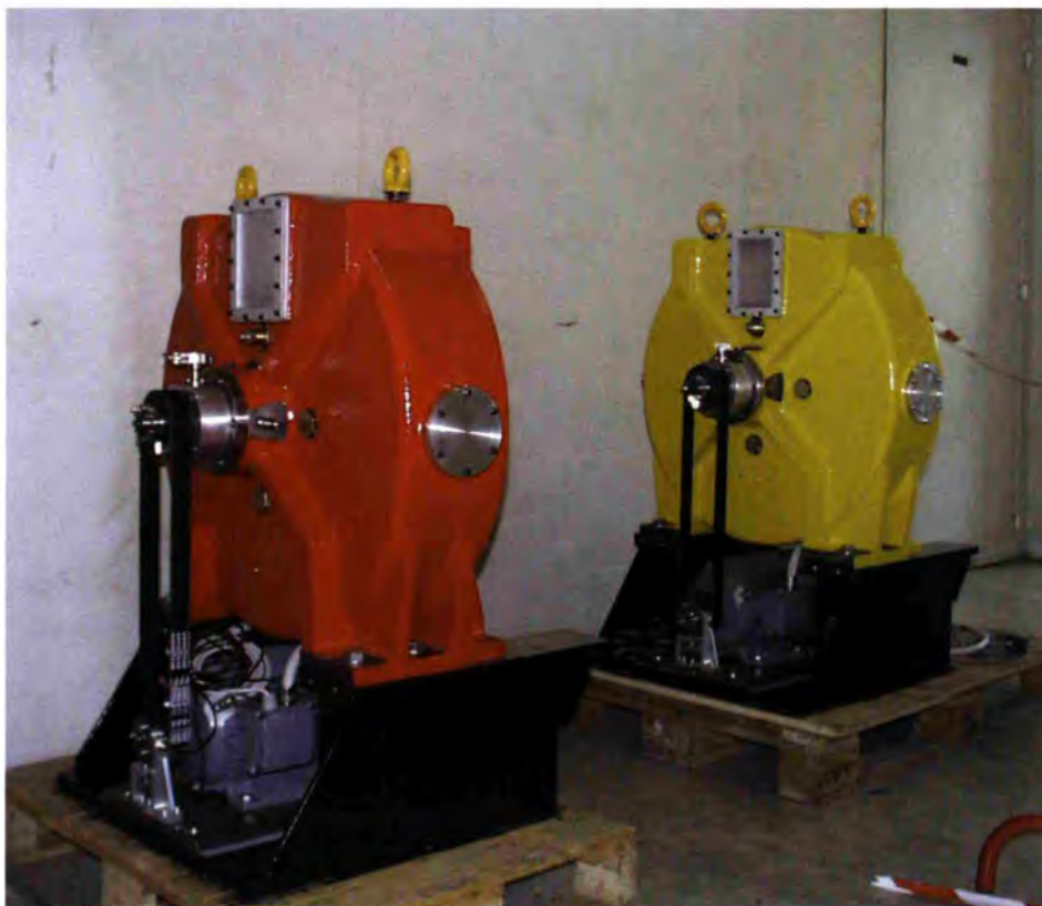
The new wheel choppers of IN4 (maximum speed: 5500 rpm).
