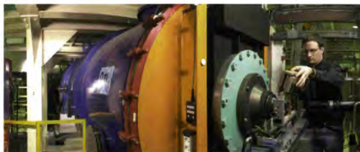
Johannes Zipfel mounting the high-temperature sample changer on D11.
