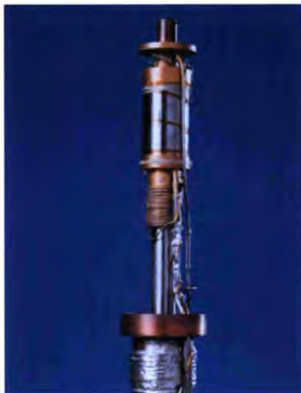
Figure 1: Picture of the Joule-Thomson stage of the XMAS cryocooler.
