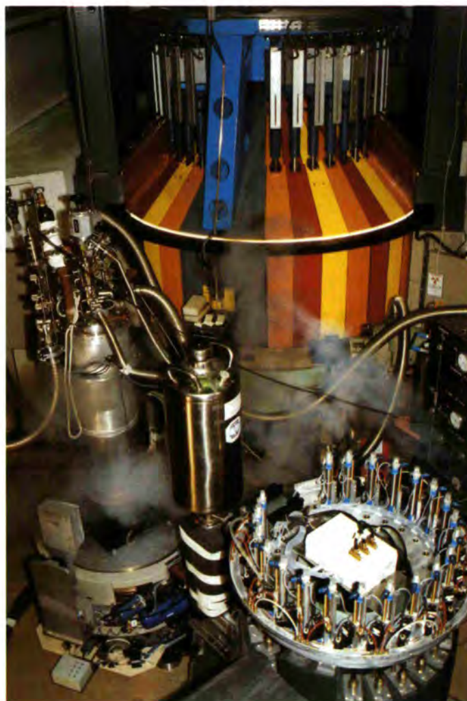
Birth of the new triple-axis spectrometer IN14 at the horizontal cold source.
