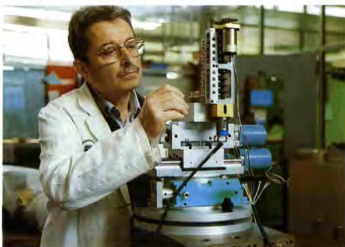
Final tests and alignment of the monochromator assembly for IN10C in collaboration with the mechanics workshop.
