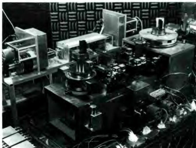
View of the central part of the GAMS4 spectrometer. The \gamma -beam originates from the left side in the picture. It is diffracted by two Si-crystals which share the axis of rotation of the two angle interferometer arms. The crystal on the right side shares additionally the rotation axis of a 24 sided polygon which allows - in conjunction with an autocollimation system - the absolute angular calibration.
