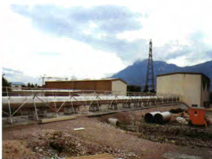
Part of the flight path for the n\bar{n} experiment. It leaves the second guide-hall (left of the picture) and enters into the detector hall (on the right).
