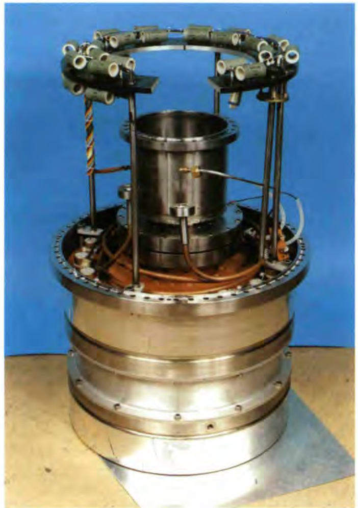
Bottom part of the super-conducting magnet for 3-axis spectrometers (Max. field: 6 Tesla, temperature range 1.5\text{ K} < T < 300\text{ K} ).
