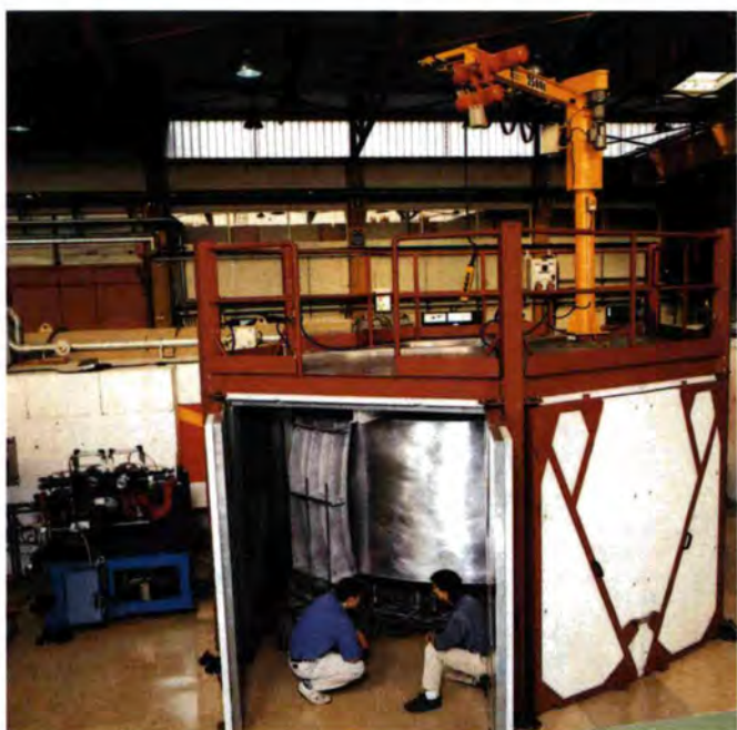
Outside view of the new backscattering spectrometer IN10C, showing the mobile shielding with working platform and crane on top. Inside the instrument you can see one He-flight box and an analyser from its rear side. Left in the picture is the Doppler drive attached to the instrument.
