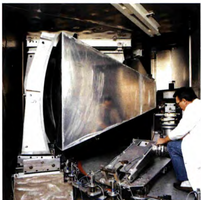
Inside view of IN10C from the small-angle analyser side. Behind René Rebesco the sample table with goniometers and the graphite deflector-chopper, on the left hand side an analyser and a Helium flight box can be seen.
