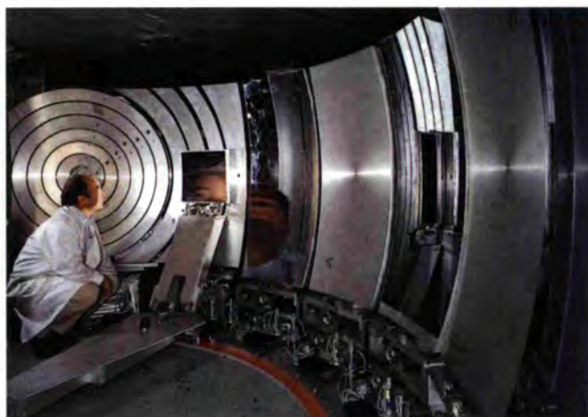
Inside view of the new backscattering spectrometer IN10C with Yvon Blanc looking at the Si(111) analysers. The left eye of Yvon is mirrored by the mobile analyser, the right eye by one of the finished large angle analysers. One can also see the goniometers on which the analysers are mounted and the pneumatic automation needed to branch the analysers to the platform, by remote handling from outside.
