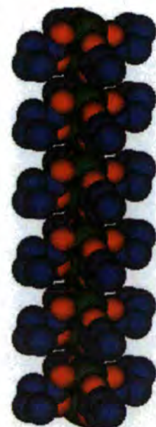
Fig. 3(college 9b box): Modelisation of the aggregate (molecular wire) for a \text{Cu}_2\text{-L4} derivative chosen instead of \text{Cu}_2\text{-S8} for sake of clarity. For \text{Cu}_2\text{-S8} the polar core is very much embedded in the ramified hydrophobic tails. Atoms : copper (green), oxygen (red), carbon (blue). Length scale : Van der Waals diameter of the carbon atom is 1.57\text{\AA} .
