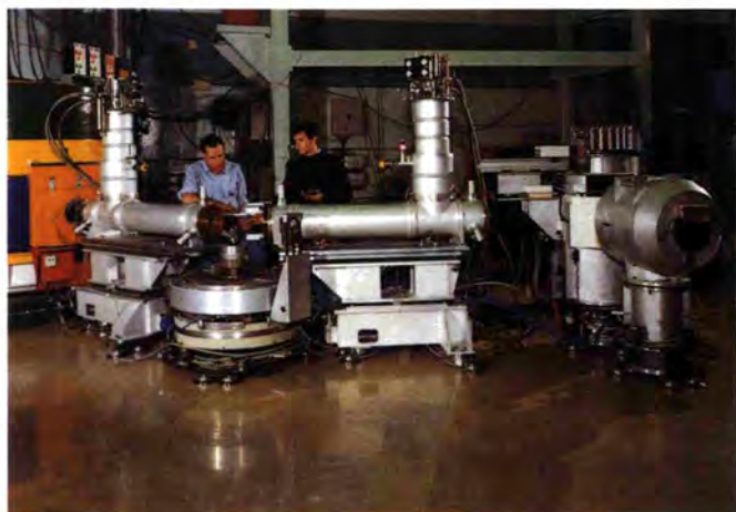
The new superconducting spin-echo magnets (see text in the 3-axis group section), installed for final testing on the host IN20 spectrometer. These optimized precession coils are expected to boost the energy resolution by several orders of magnitude.
