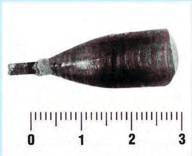
Fig. 1: Optical micrograph of a single grain of the AlPdMn icosahedral quasicrystal obtained via Czochralski growth (scale in cm).
