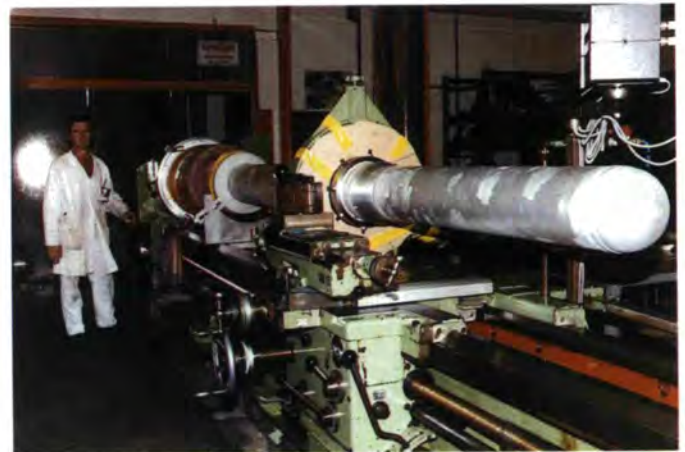
Fig. 9: Marc Locatelli in the ILL workshop reshaping a beamtube thimble.
