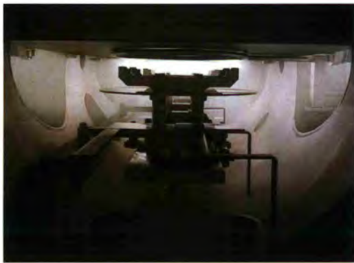
DPT - Fig. 12: A view inside the deposition chamber with an Argon plasma illuminating the substrate carrier. See report p. 137.
