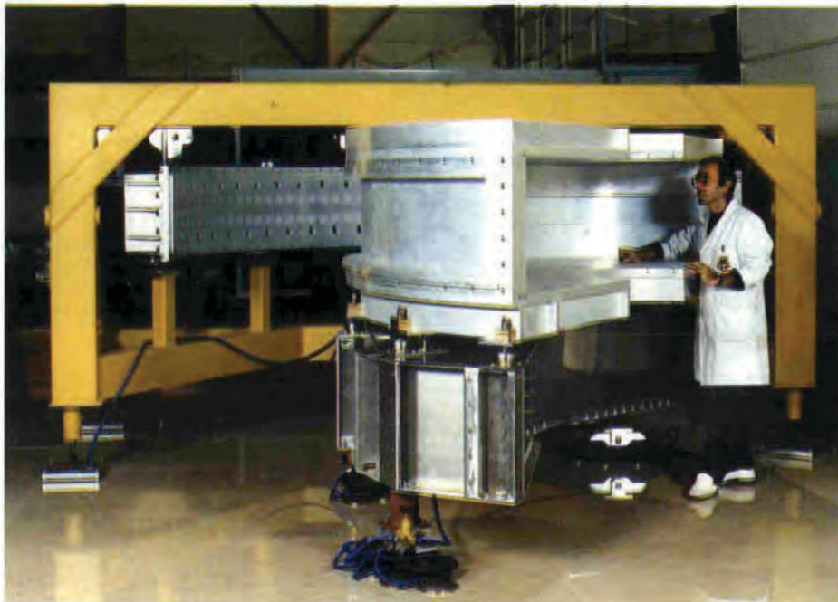
DPT - Fig. 3: The housing of the D20 banana multidetector opens in two pieces: Michel Berneron stands at the side of the front part on the final aluminium support which will be used at D20 on a 'Tanzboden'; the back part is mounted on a special strong support (yellow) used during the construction phase for the mounting of the 50 glass plates composing the 1600 cells, for their precise adjustment and for the operation of closing the housing. See report p. 129.
