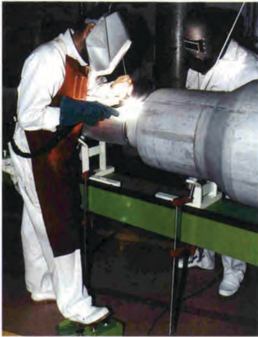
Fig. 10a: J.P. Gonella and his colleague J.F. Garin-Cuchet welding a beamtube thimble.
