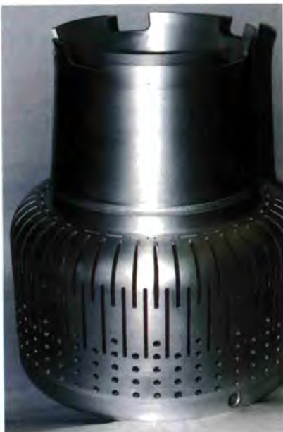
Fig. 7: The turned-down grid for the new vessel.
