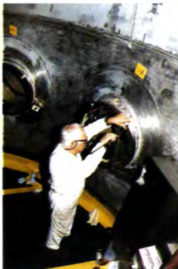
Fig. 17: F. Müller verifying the dimensions of a beam tube in the reactor swimming pool.
