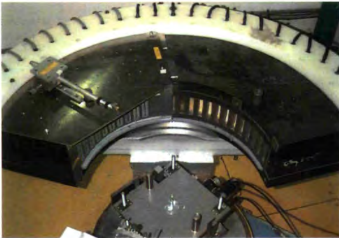
DS - DIF - Fig. 1: New 25-collimator detector covering 150° on DIA. See report p. 120.
