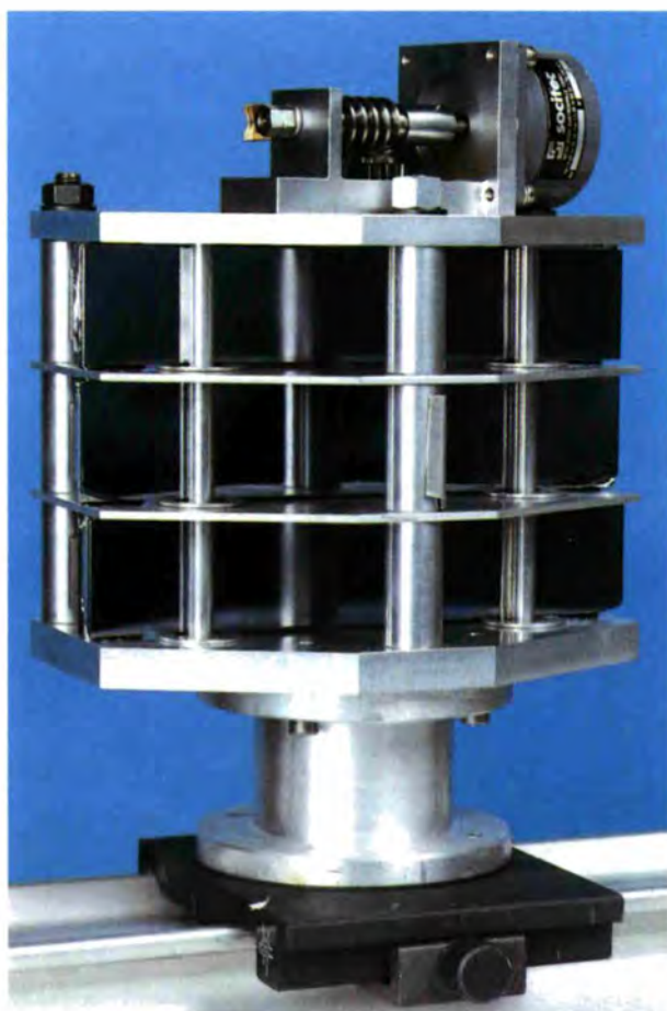
DS - TAS - blue box - Fig. 2: Photograph of the new IN20 analyser using elastically bent Si 111 crystals. Each of the three stages contains a pack of three silicon plates; the plates in the top and bottom part are skew cut with an inclination angle of 7.5° to provide fixed vertical focusing optimised for k_f = 2.66 \text{ \AA}^{-1} . See report p. 133.
