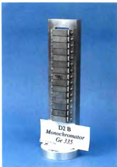
DPT - Fig. 7: The final assembled germanium monochromator for D2B. See report p. 155.
