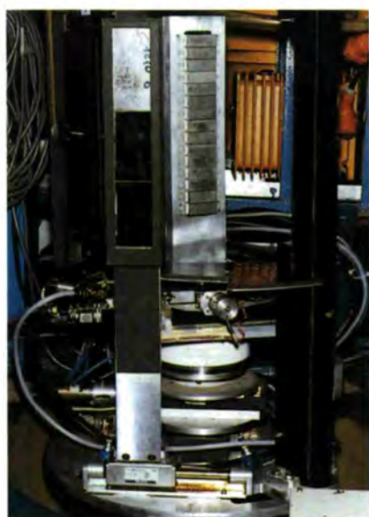
DS - DIF - Fig. 5: The new D2B monochromator, with the large graphite filter for work at 2.4 Å. See report p. 121.
