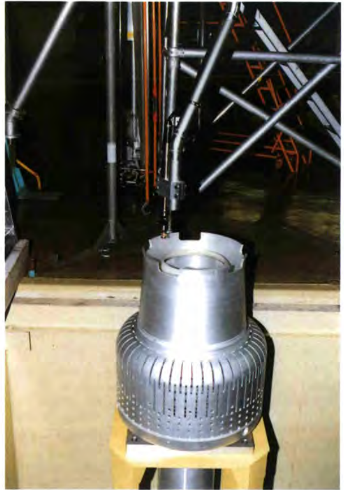
Fig. 2: Preparing the inspection of the new «turned-down» grid.
