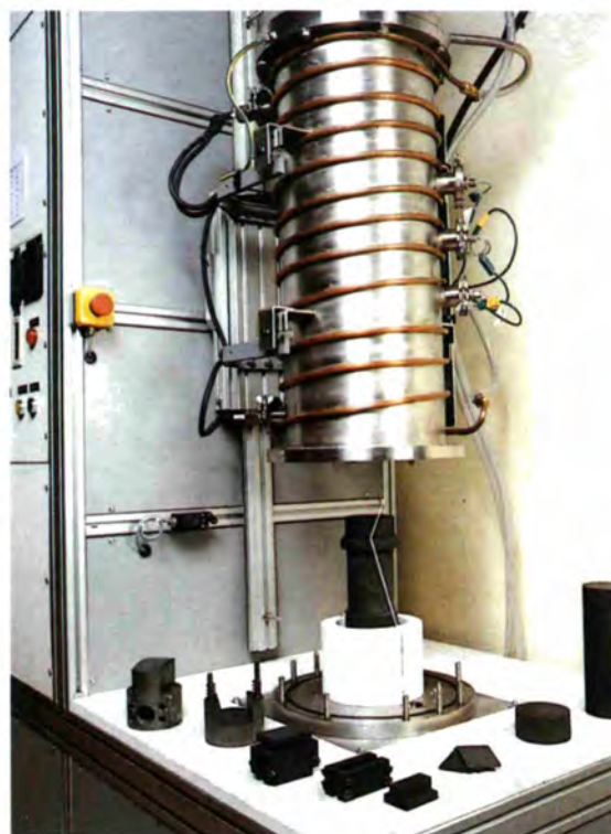
DPT - Fig. 6: The new hot press developed by B. Guerra and used for bending the Germanium wafers for the D2B monochromator. The design ensures a uniform temperature region of 200 mm high up to 900 °C, and pressures up to 3.5 bars during a fully automated cycle. See report p. 155.
